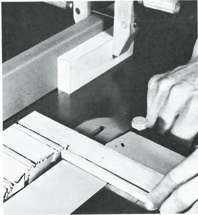
Fig. 14-24. Using clearance block to cut duplicate parts.
