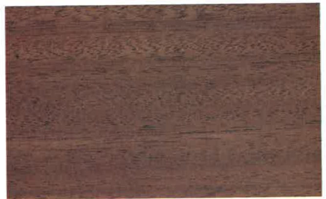
MAHOGANY, AFRICAN. Characteristics are similar to American varieties. Slightly coarser texture and more pronounced grain patterns. Quarter sawing or slicing produces a ribbon grain effect (as shown). Source: Ivory Coast, Ghana and Nigeria. Used for fine furniture, interior finish, art objects and boats.
