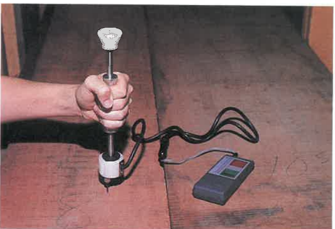
Fig. 35-13. Top. Modern digital moisture meter. LED indicates correct moisture percentage. Middle. Probes inserted into end cut. Bottom. Hammer probe provides readings up to 1 in. below the surface. (Forestry Suppliers, Inc.)
