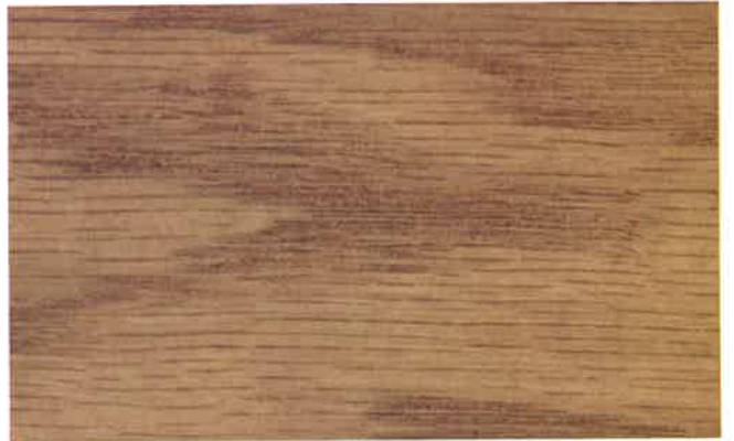
OAK, WHITE. Heavy (47 lbs. to cu. ft.), very hard, durable, and strong. Works best with power tools. Heartwood is greyish-brown with open pores that are distinct and plugged with a hairlike growth called tyloses. Used for high quality millwork, interior finish, furniture, carvings, boat structures, barrels and kegs.
