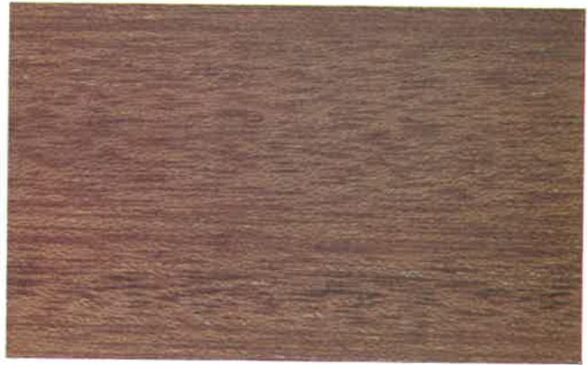
MAHOGANY, PHILIPPINE. Medium density and hardness (37 lbs. to cu. ft.). Open grain and coarse texture. Works fairly well with hand or machine tools. Varies in color from dark red (Tanguile) to light tan (Lauan). Used for medium price furniture, fixtures, trim, wall paneling. Also, boat building and core stock in plywood.
