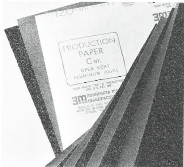
Fig. 11-6. Typical abrasive paper markings. Light toned sheets are open coated; dark sheets are closed coated.
