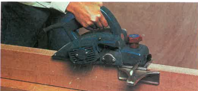
Fig. 3-9. This operator is using the proper procedure to plane a surface with a portable electric plane. (Makita U.S.A., Inc.)
