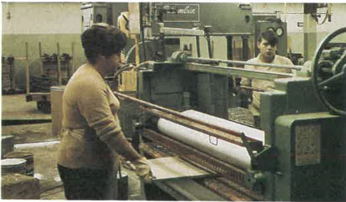
Fig. 9-40. This glue spreader applies adhesive to both the top and bottom surfaces of edge-glued lumber core stock. Eventually it will be bonded with veneer or high pressure decorative plastic laminate. (Black Brothers)
