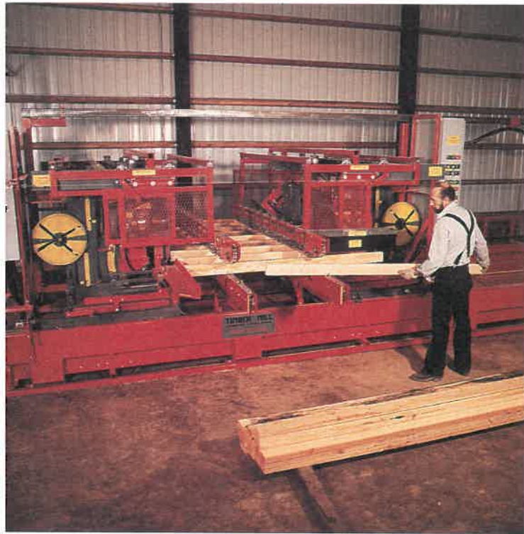
Fig. 14-85. Basic double end sawing machine. Space between sawing heads is adjustable for various widths of material. (Speed Cut, Inc.)
