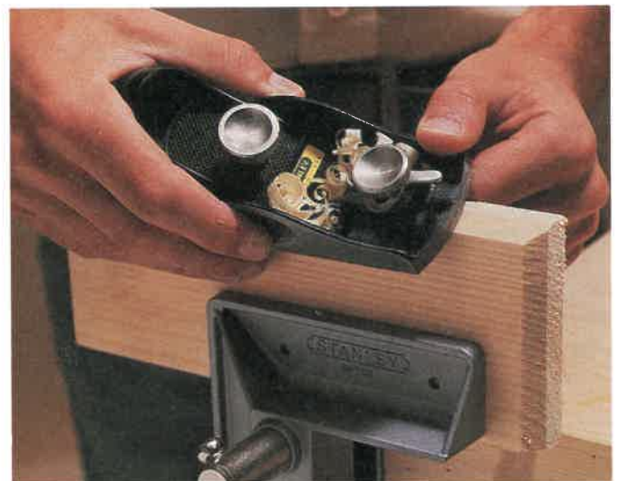
Fig. 8-28. Top. Laying out a chamfer. Bottom. Planing a chamfer. (The Stanley Works)
