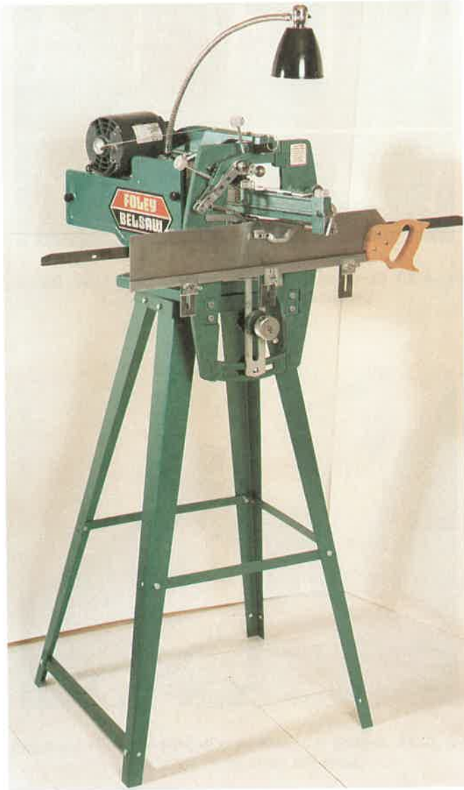
Fig. 4-25. Automatic saw filer. After each file stroke, pawl engages teeth and moves blade into position for the next stroke. (Foley-Belsaw Co.)
