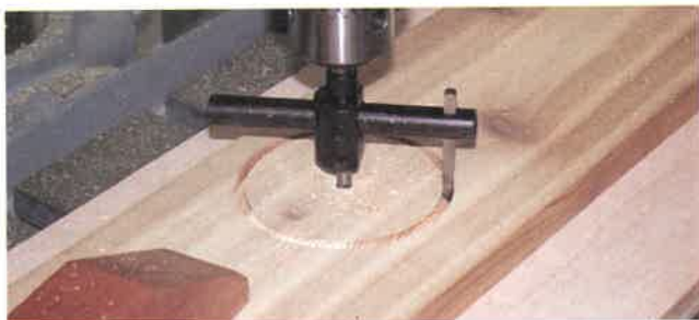
Fig. 3-22. The fly cutter is a dangerous tool. Be sure to clamp the work securely to the table when using this tool.
