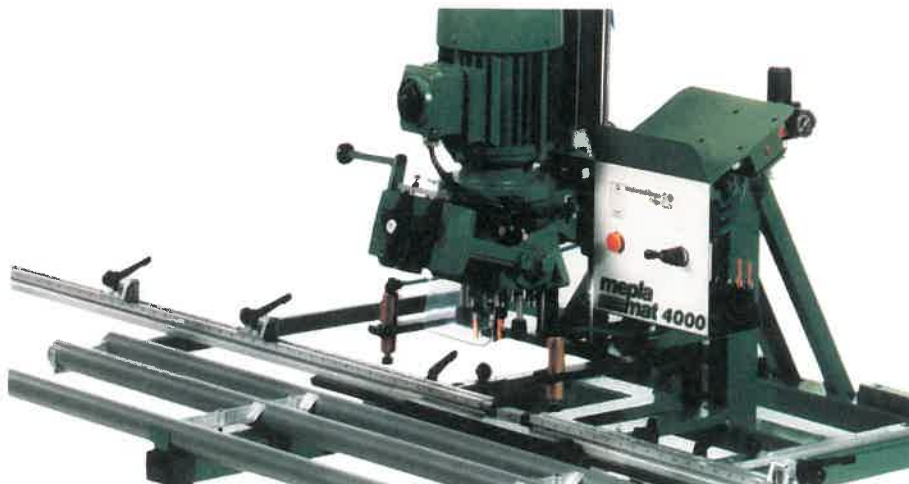
Fig. 21-16. 32mm equipment with a 12-spindle boring head and "calibrator-fence" system. (Mepla, Inc.)
