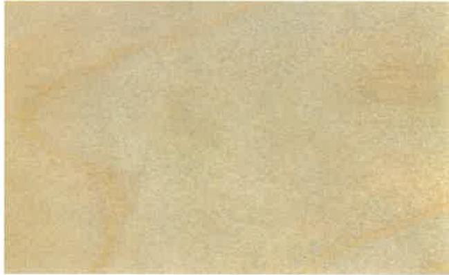
BIRCH, WHITE. Selected sapwood rotary-cuttings of regular birch veneer. Same characteristics as birch except nearly white in color. Used to make plywood for installations requiring a very light, fine textured material.
