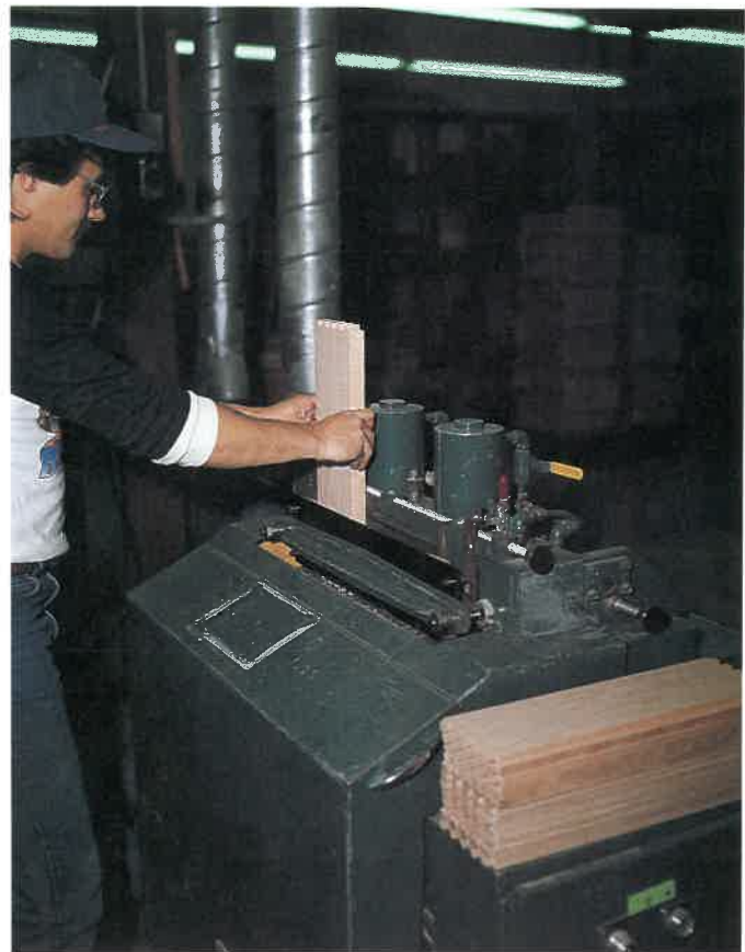
Fig. 36-6. Semiskilled worker feeds workpieces into double-end tenoner. (Campbellrhea Mfg., Inc.)
