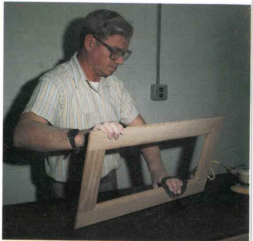
Fig. 11-24. Final sanding before finish is applied. (Campbellrhea Mfg., Inc.)
