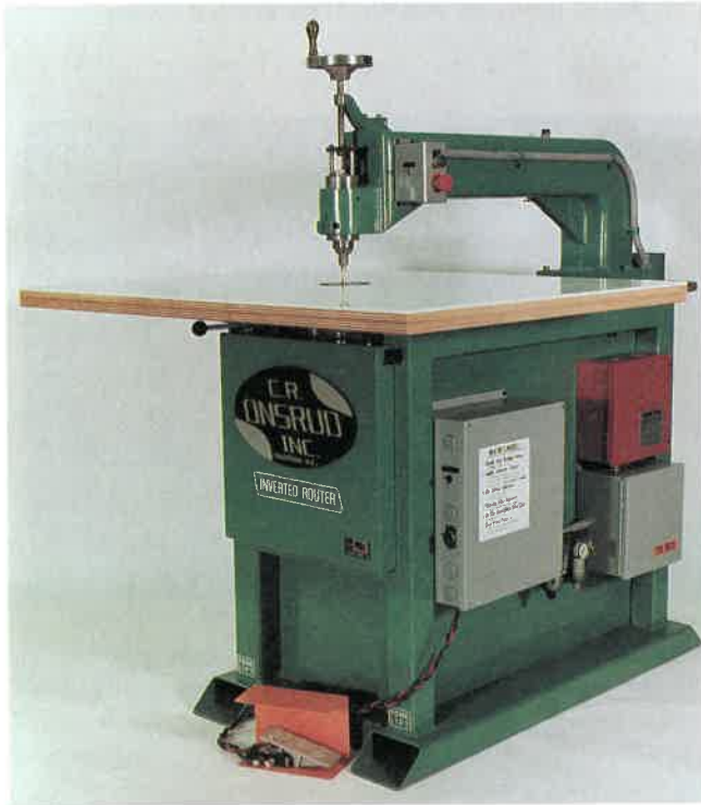
Fig. 18-25. Inverted pin router has the cutter mounted below the table with the pin in the arm above. (C.R. Onsrud, Inc.)
