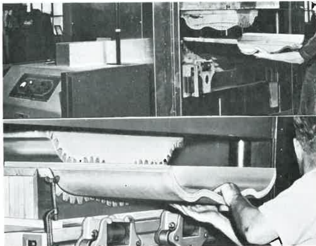
Fig. 9-43. Top. High frequency press with 30 kW generator. Dies are made of wood with a metal face that serves as the electrode. Press is closed and pressure applied by hydraulic power. Bottom. Removing finished panel, which will be used for serpentine drawer fronts. (Lodge and Shipley Co.)
