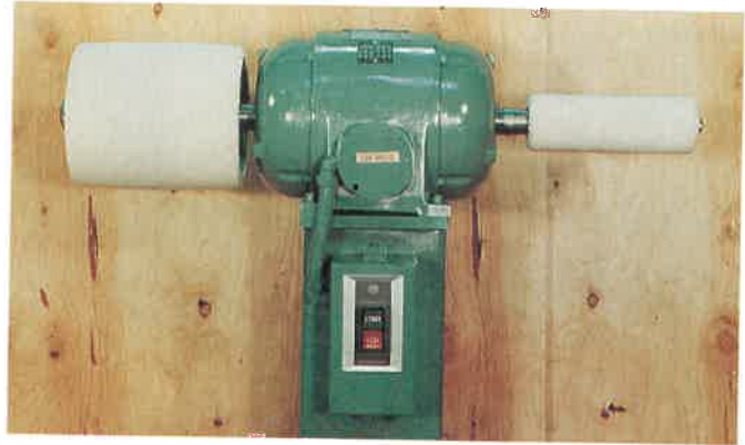
Fig. 19-35. This two-spindle drum sander can be used to sand curved pieces. (Ekstrom, Carlson and Co.)
