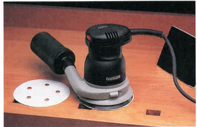
Fig. 19-24. Top. An example of a right-angle random orbit sander. (Porter-Cable) Bottom. An example of an in-line random orbit sander. (Woodcraft Supply Corporation)
