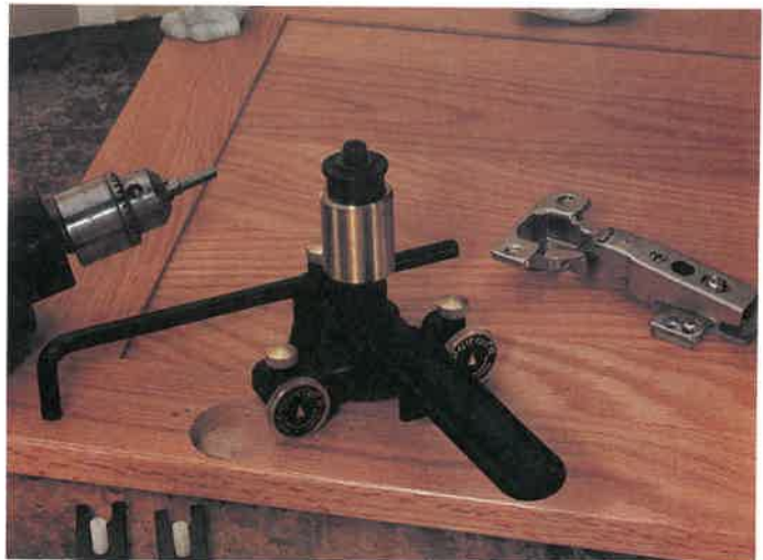
Fig. 21-14. Shelf-drilling jig eliminates the time-consuming layout work usually associated with installing shelf supports. Right. A hinge-boring jig used for drilling 35mm holes for cup hinges. (Veritas Tools, Inc.)
