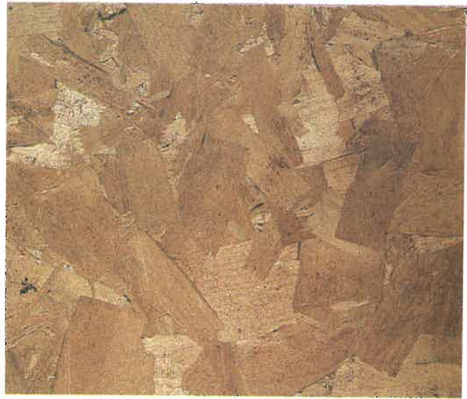
Fig. 2-18. Waferboard consists of multilayers of wood wafers, bonded together under extreme heat and pressure with a water-proof phenolic resin. The result is a rigid, flat panel, dimensionally stable and equally strong in all directions. It may be used as an interior or exterior material. (Georgia Pacific Corporation)
