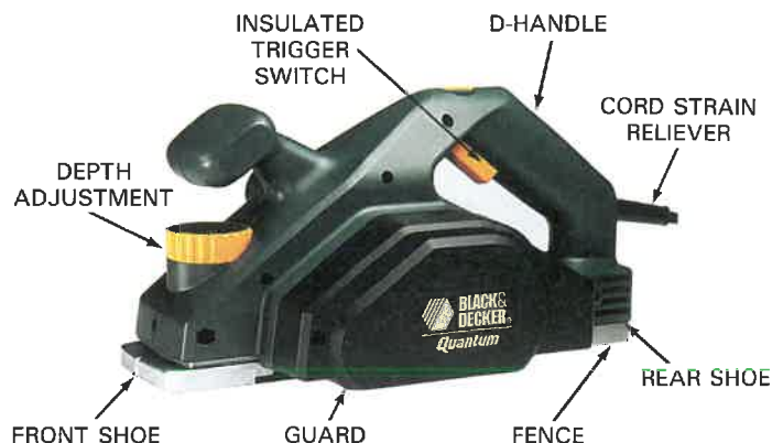
Fig. 13-22. Parts of an electric plane. (Black & Decker)
