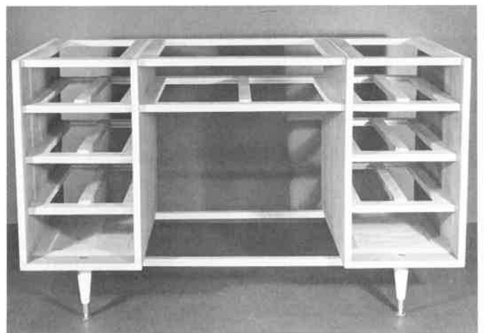
Fig. 21-30. Basic assembly of a kneehole desk. The bottom brace strips are removed after back panels and top are attached. (John Moeller)
