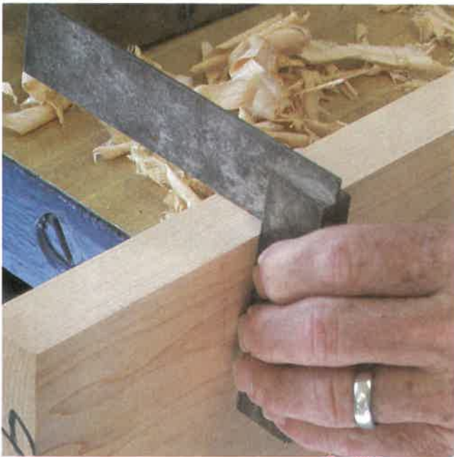
Fig. 5-17. Checking the edge to see that it is square with the face.
