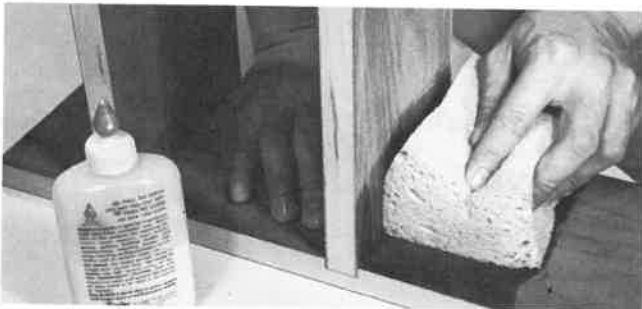
Fig. 9-32. Cleaning a glue joint with a sponge moistened with hot water.
