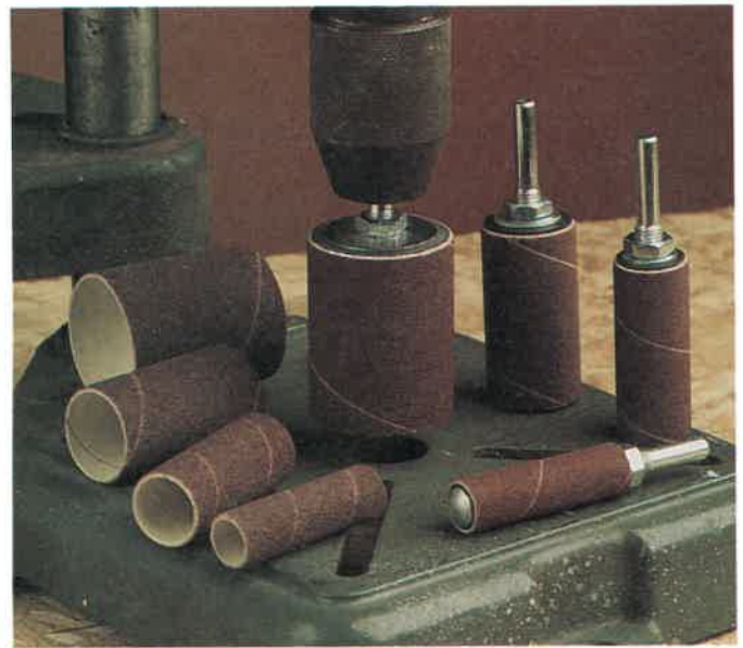
Fig. 16-27. Sanding drums are ideal for sanding curved pieces on the drill press. A variety of sizes are available. (Leichtung, Inc.)
