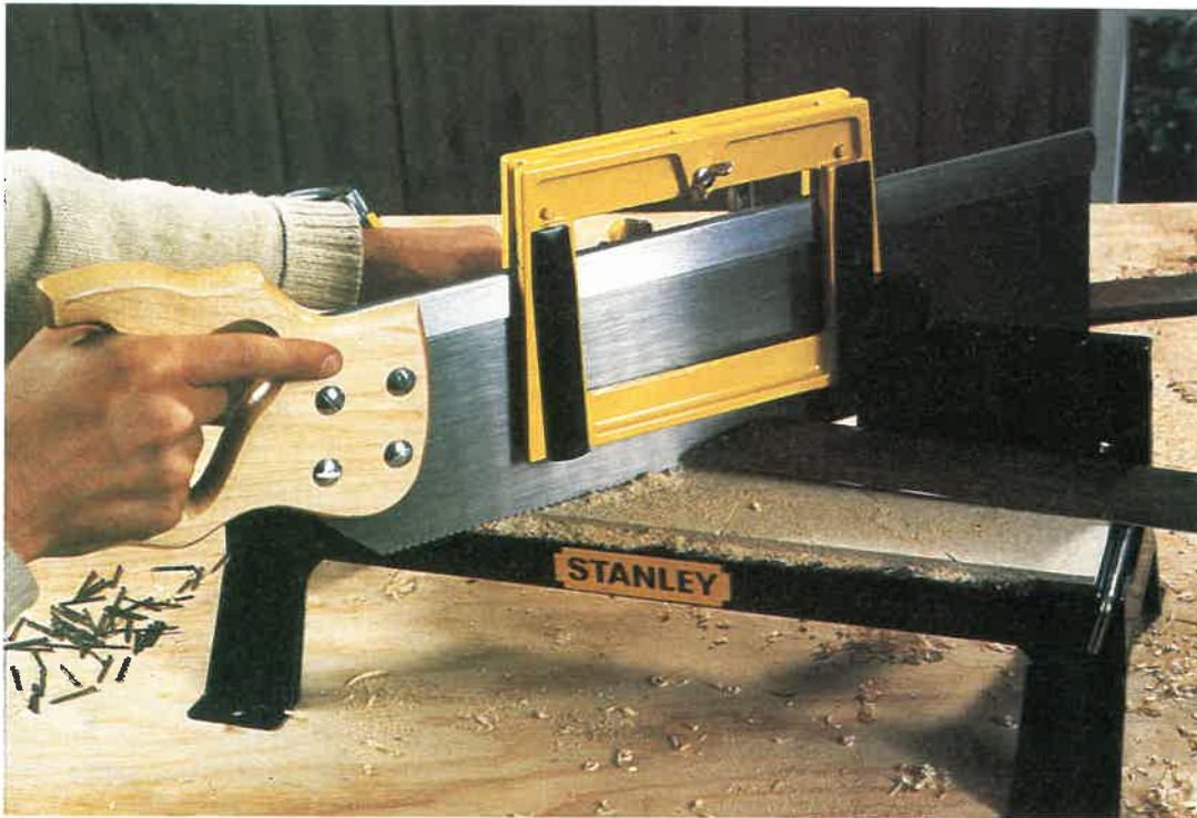
Fig. 5-29. The miter box will produce very accurate cuts at angles up to 45 degrees. (The Stanley Works)
