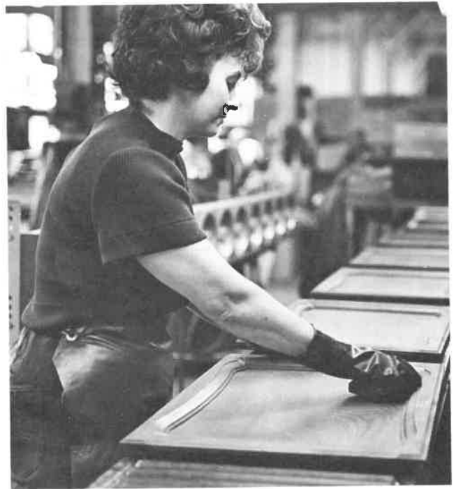
Fig. 12-81. Hand rubbing kitchen cabinet doors that are carried on free-turning rollers. (International Paper Co.)
