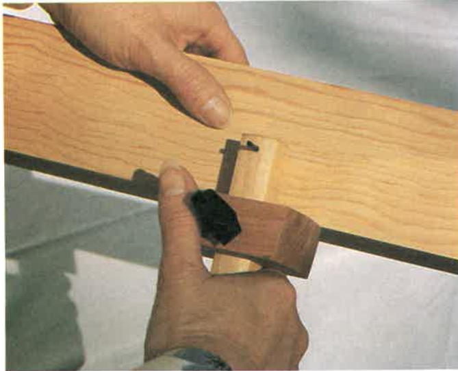
Fig. 5-13. Using a mortise gauge to lay out stock thickness.
