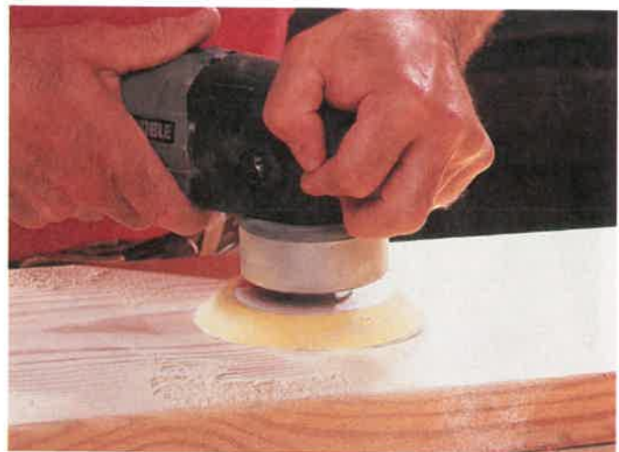
Fig. 19-2. Using a portable random orbit finishing disk sander to smooth a surface. (Porter-Cable Corporation)
