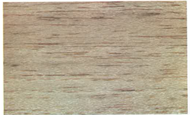
BALSA. The lightest wood available (12 lbs. to cu. ft.). Very soft and easily cut with knives. Best known for its use in model aircraft construction. Also used for life rafts, duck decoys, hat blocks, and other lightweight items. Chief source is Ecuador.
