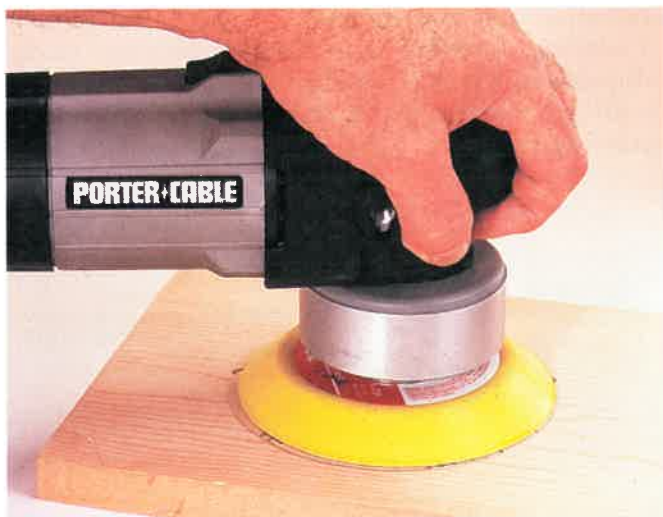
Fig. 19-23. A random orbit sander being used to perform finish sanding. (Porter-Cable)
