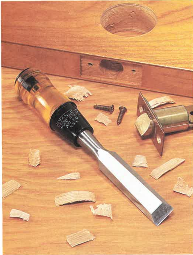
Fig. 3-2. This sharp chisel is the proper tool for the installation of the lock set. It is very sharp, so use it with care. (The Stanley Works)
