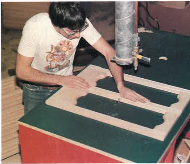
Fig. 36-7. Semiskilled assembly line worker routing a groove on the back side of a cabinet door frame. This task requires limited on-the-job training. (Bertch Wood Specialties)
