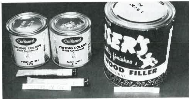
Fig. 12-12. Colors in oil on the left can be used to color paste filler on the right.
