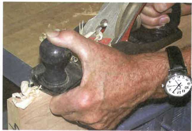
Fig. 5-18. Guiding the toe of the plane with fingers held on the plane bottom. Used for a fine and accurate cut.
