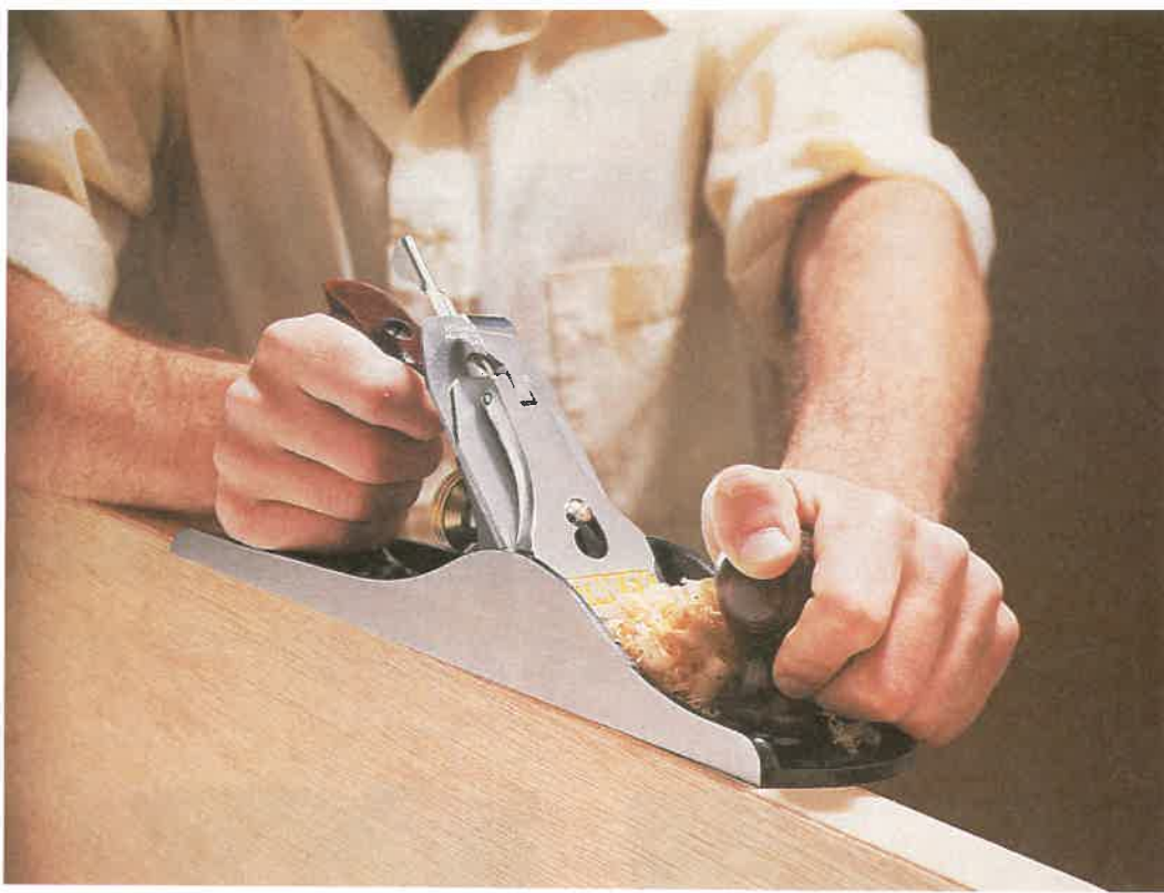
Fig. 5-16. Try to produce a smooth, true edge with as little planing as possible. (The Stanley Works)
