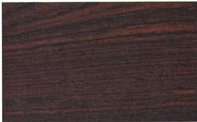
COCOBOLA. Dense, hard and oily. A difficult wood to work because of an interwoven grain. Bright red when freshly cut, but soon darkens. Source: Central America. Used for fancy cabinetwork and knife handles.
