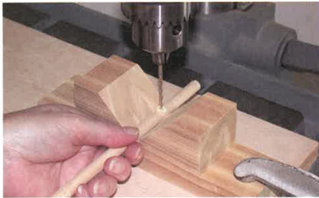
Fig. 3-21. Using a V-block to drill a hole in round stock is a safe practice.
