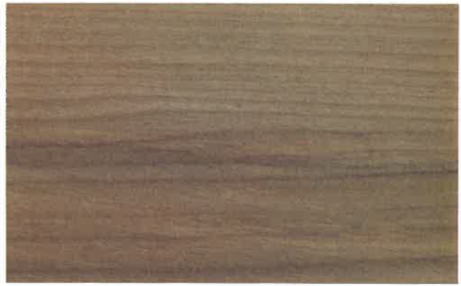
BIRCH. A hard, strong, wood (47 lbs. to cu. ft.). Works well with machines and has excellent finishing characteristics. Heartwood, reddish-brown with white sapwood. Fine grain and texture. Used extensively for quality furniture, cabinetwork, doors, interior trim, and plywood. Also used for dowels, spools, toothpicks, and clothespins.
