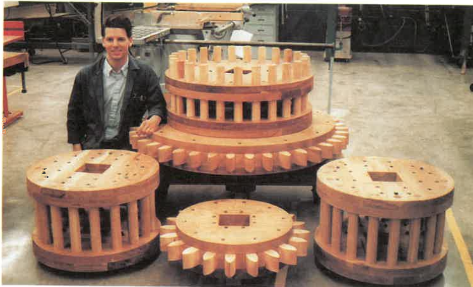
These custom wooden gears were designed and fabricated for use in an authentic grist mill restoration project in Vigo County, Indiana. The gear bodies are white oak and the teeth are hard maple. (Mark Clauss)
