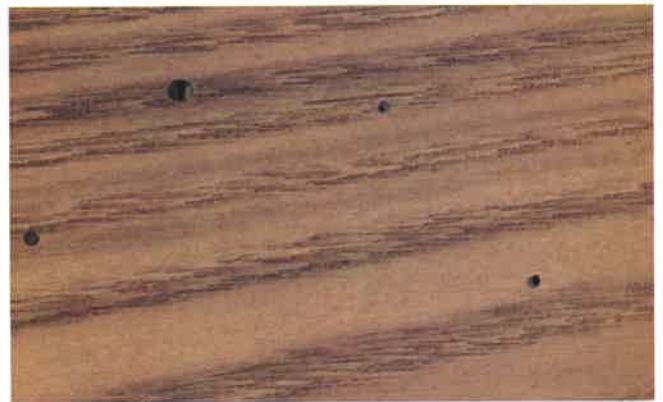
CHESTNUT. Coarse textured, open grain, and very durable. Reddish brown heartwood. Easily worked with hand or machine tools. Source: Eastern United States. Available only in a wormy grade due to the "chestnut blight."
