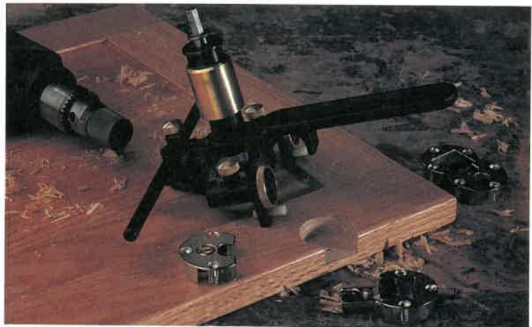
Fig. 21-15. Right. Drilling 35mm flap hinges. Left. Drilling standard 35mm hinges. (Veritas Tools, Inc.)
