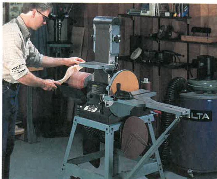
Fig. 19-16. Combination disk and belt sander attached to a dust collector. (Delta International Machinery Corp.)
