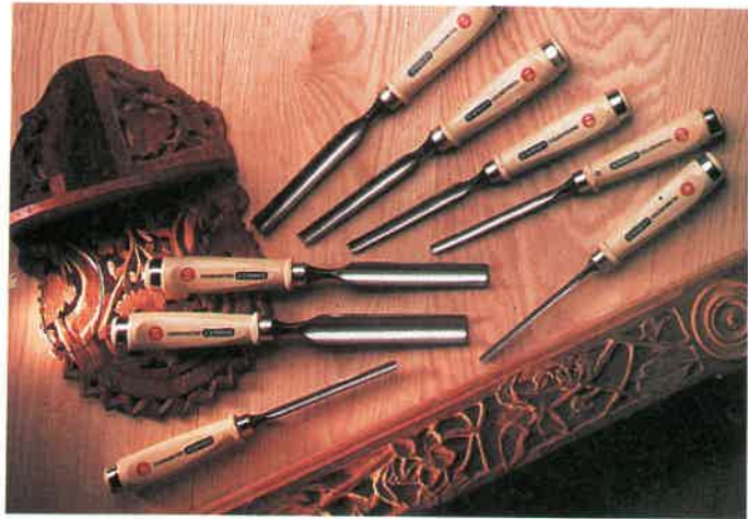
Fig. 20-13. Top. Carving tools commonly used for relief carving. Bottom. Gouges are used for general shaping. (Stanley Tools)
