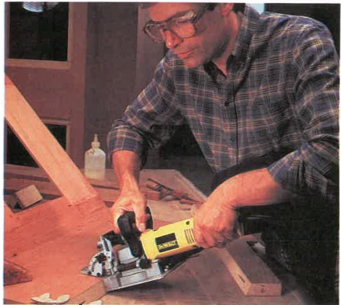
The plate joiner is firmly held with both hands and safety glasses are worn to provide maximum safety. (DeWalt)
