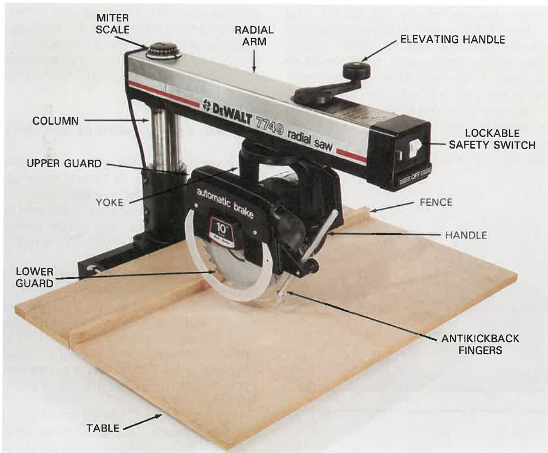
Fig. 14-59. Parts of a 10 in. (254 mm) radial arm saw. (DeWalt, Div. of Black and Decker)
