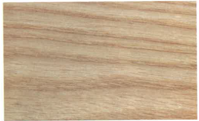
ASH, WHITE. Strong, stiff, and fairly heavy (42 lbs. to cu. ft.). Works fairly well with hand tools but splits easily. Heartwood is a pale tan with a texture similar to Oak. Used for millwork, cabinets, furniture, upholstered frames, boxes and crates. Used extensively for baseball bats, tennis rackets, and other sporting equipment.
