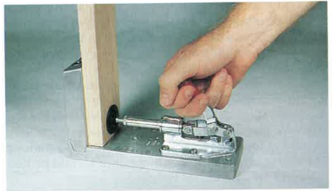
Fig. 9-22. Toggle clamps are now being widely used by woodworkers to hold workpieces in jigs and fixtures and for typical machining operations. (Kreg Tool Company)
