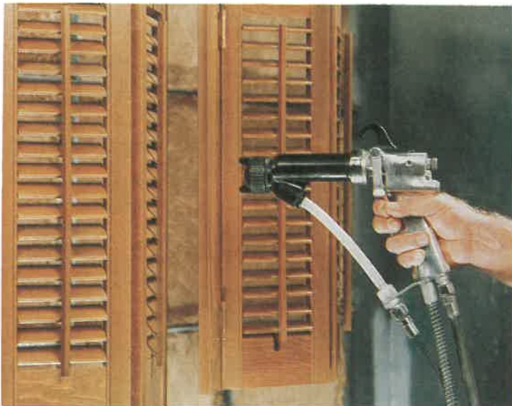
Fig. 12-68. On this production line, the final coat of lacquer is supplied through a hose. (Ransburg Electrostatic Equipment)
