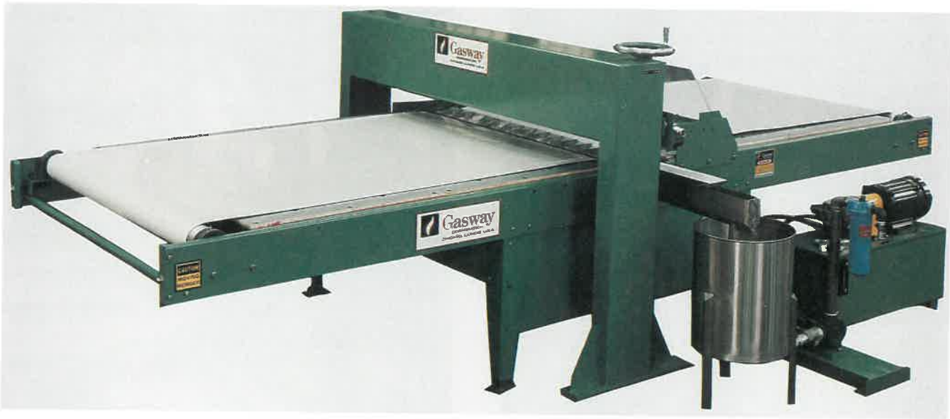
Fig. 12-78. Modern curtain coating machine. Conveyor belt speeds are adjustable from 100 to 450 fpm (30.5 to 137 mpm). (Gasway Corp.)
