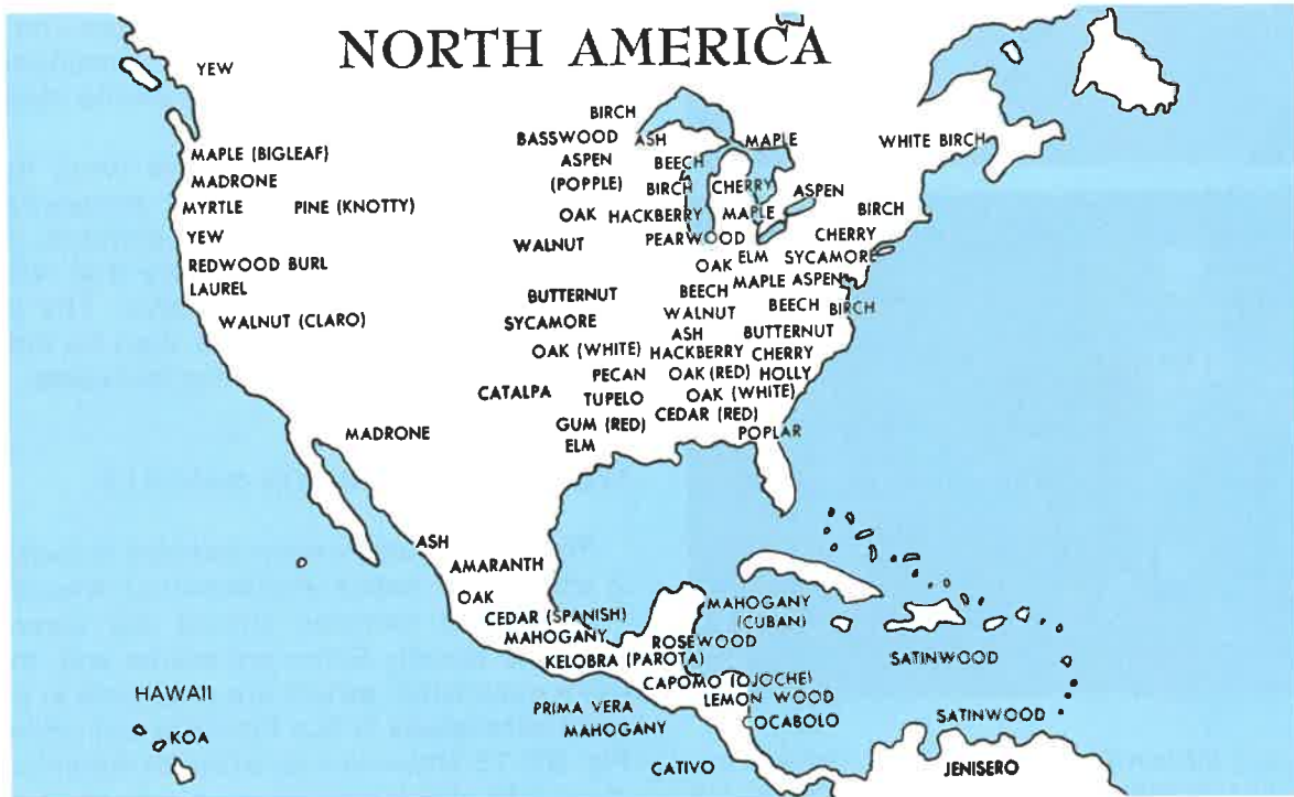
Fig. 35-16. Hardwoods of North America and where they grow. (Fine Hardwoods-American Walnut Association)
