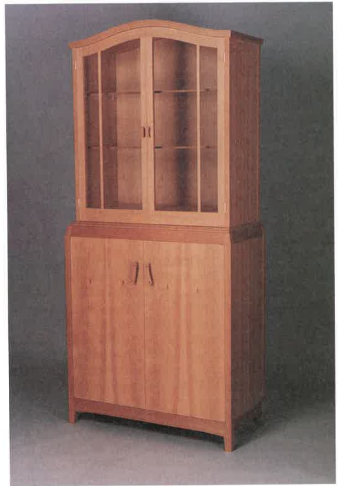
Fig. 21-4. This china cabinet is an example of carcass construction. Notice the framed glass panel doors covering the shelves. There are drawers behind the lower doors. (David Welter)
