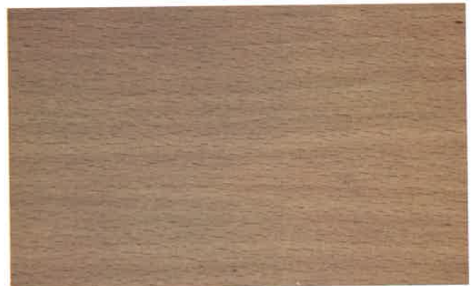
BEECH. Heavy, hard and strong. (44 lbs. to cu. ft.) A good substitute for Sugar Maple but somewhat darker in color, with a slightly coarser texture. Used for flooring, furniture, brush handles, food containers, and boxes and crates.
