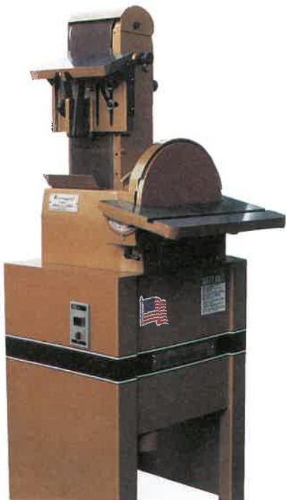
Fig. 19-8. Stationary belt sander. Sanding unit can also be turned to a horizontal position and other angles. Belt is 6 in. (152.5 mm) wide. (Powermatic)
