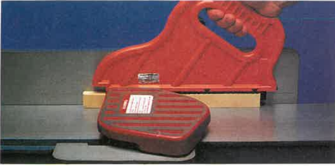
Fig. 3-8. This operator is using a pusher block to surface a short piece of stock. (CMT Tools)
