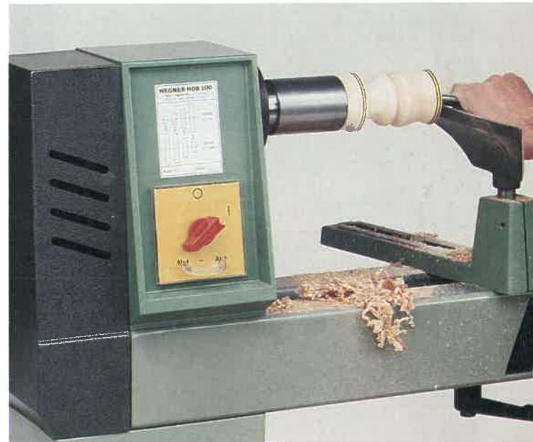
Fig. 17-42. The speed chuck may be used to hold small turnings on one end for both internal and external machining. (AMI, Ltd.)
