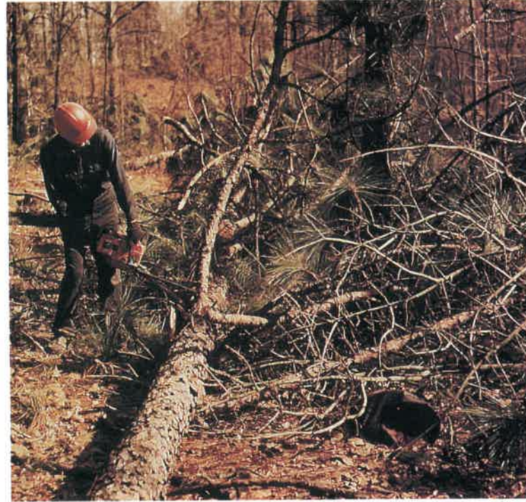
Fig. 35-21. Removing the limbs and top with a chain saw. The log will then be cut into suitable lengths for transport to the mill. (Southern Forest Products Association)
