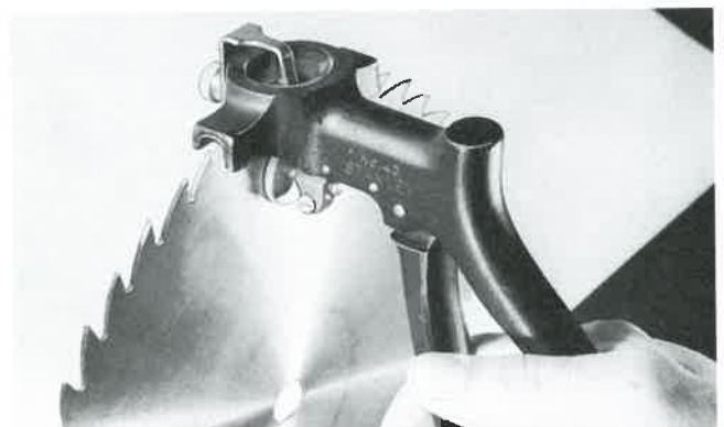
Fig. 14-52. Setting circular saw teeth with a hand set.
