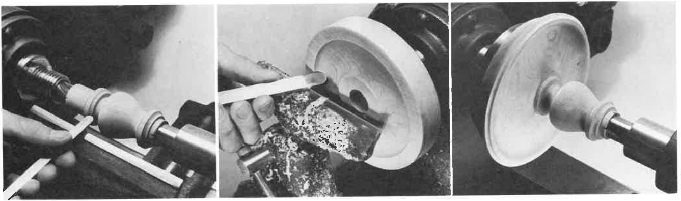
Fig. 17-34. Assembling work on the lathe. Left. Turning the stem. Center. Turning the base. Right. Parts glued and assembled.
