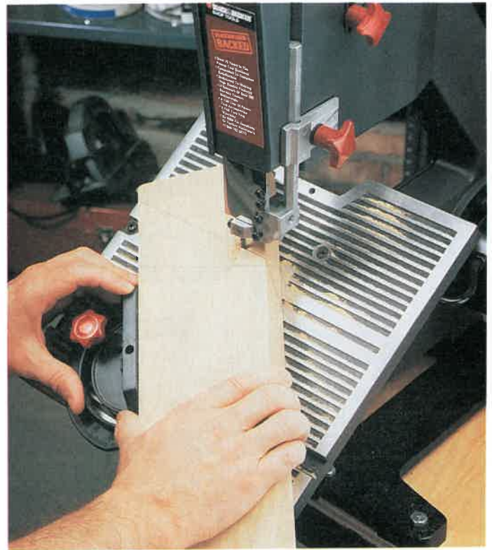
Fig. 3-17. The upper guide assembly of this band saw is properly adjusted for the thickness of stock being cut. (Black & Decker)
