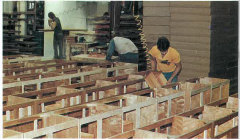
Fig. 34-1. Standardized kitchen cabinets have interchangeable parts. Drawers are installed before units are given a final inspection, then they are individually boxed for shipment. (Bertch Wood Specialties)
