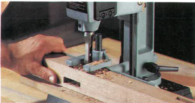
Fig. 16-23. Cutting a mortise with a hollow chisel mortiser. (Delta International Machinery Corp.)
