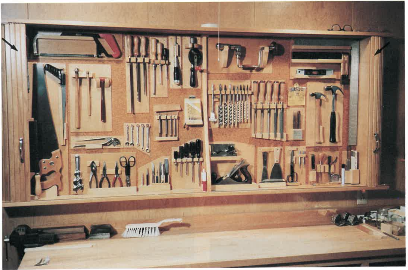
Fig. 33-21. Home workshop bench and tool panel. To close the panel, tambour sliding doors (arrows) are pulled from behind the panel to the front.
