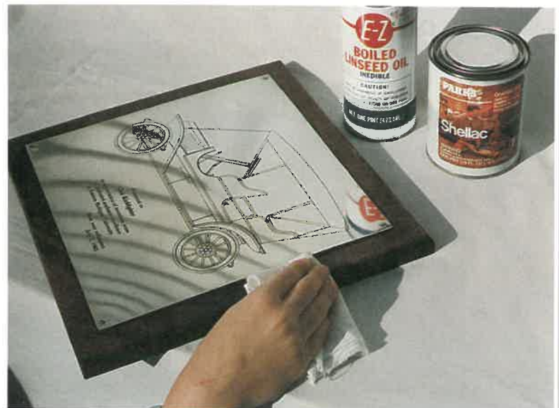
Fig. 12-24. Applying French polish with a cloth. French polish is a mixture of shellac, alcohol, and boiled linseed oil.
