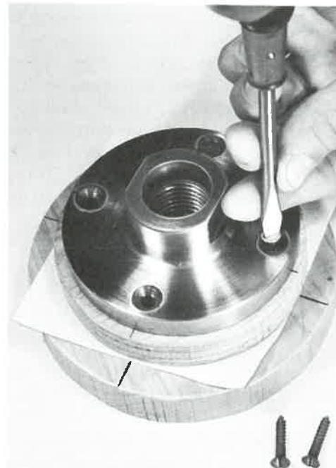
Fig. 17-28. Mounting work on a faceplate.
