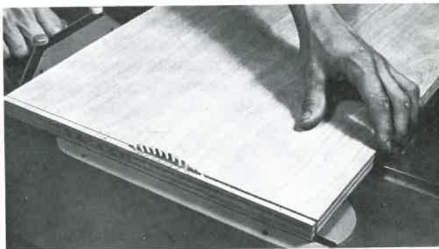
Fig. 14-25. Cutting plywood with a special blade. Guard should be used. It has been removed here to show the operation.
