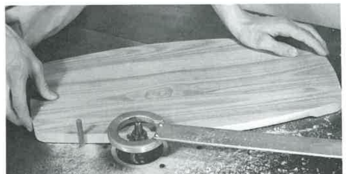
Fig. 18-40. Shaping a curved edge. Work is positioned against the starting pin. The collar controls depth of cut.
