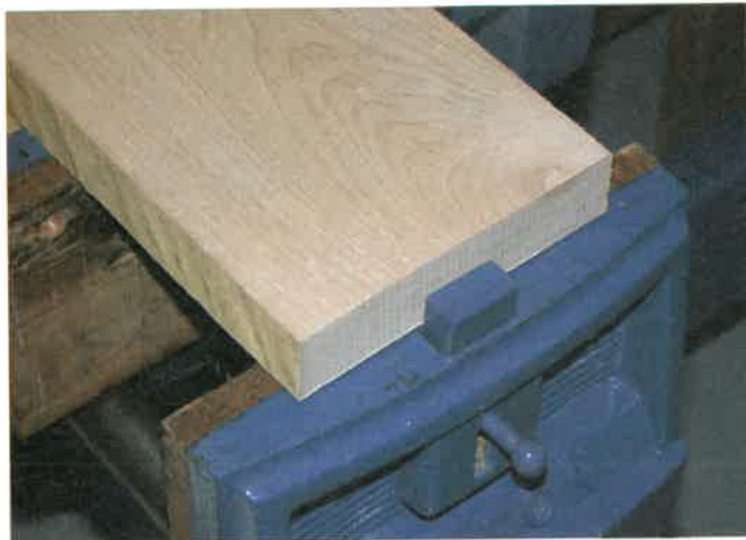
Fig. 5-14. Clamping thin pieces for planing. Keep the vise dog below the surface of the stock so it will not damage the plane.
