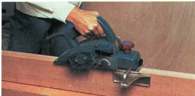
Fig. 13-24. Using a portable electric plane to trim the edge of a piece of stock. (Makita U.S.A., Inc.)
