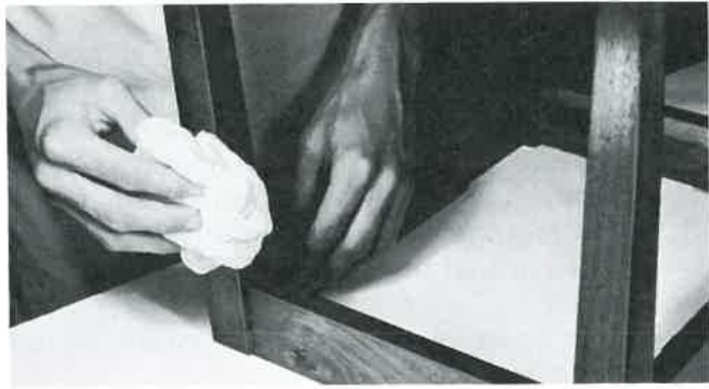
Fig. 12-39. Wiping surface lightly with a tack cloth before applying final coat.
