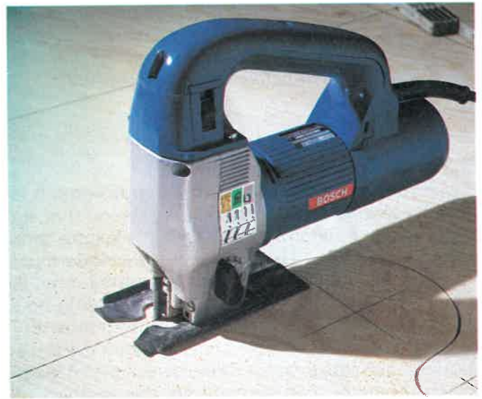
Fig. 15-38. When making a series of circular cuts with the saber saw, use a line to guide the cut. (Bosch Power Tool Corp.)
