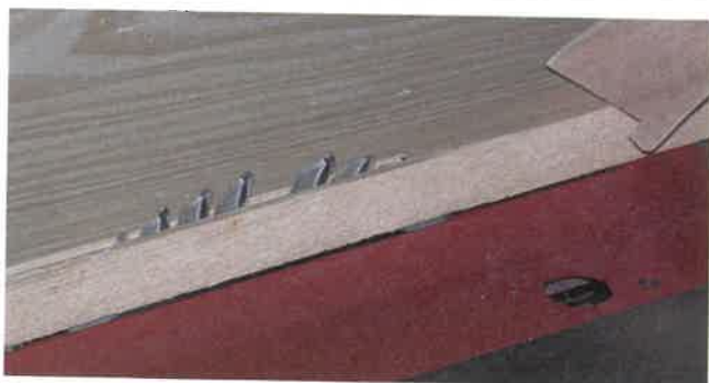
Fig. 14-16. Ripping stock to width. Top. Guard in position. Bottom. Guard and splitter removed to show operation.
