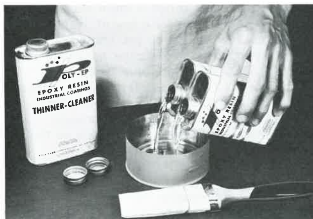
Fig. 12-35. Mixing epoxy resin. The two cans are permanently attached.
