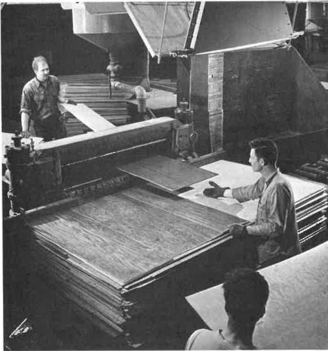
Fig. 35-32. Veneer sheets are fed through a glue spreader and placed in the "lay-up."
