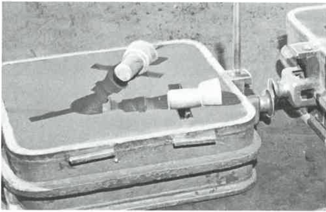
Fig. 32-16. Cores in position in the drag. Note that these particular cores are supported on only one end. (Fisher Controls)
