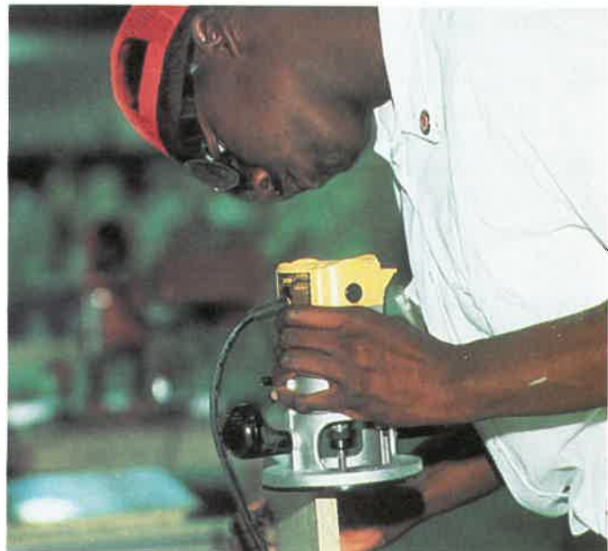
Fig. 3-5. This student woodworker is wearing proper eye protection for the operation he is performing. (VICA)
