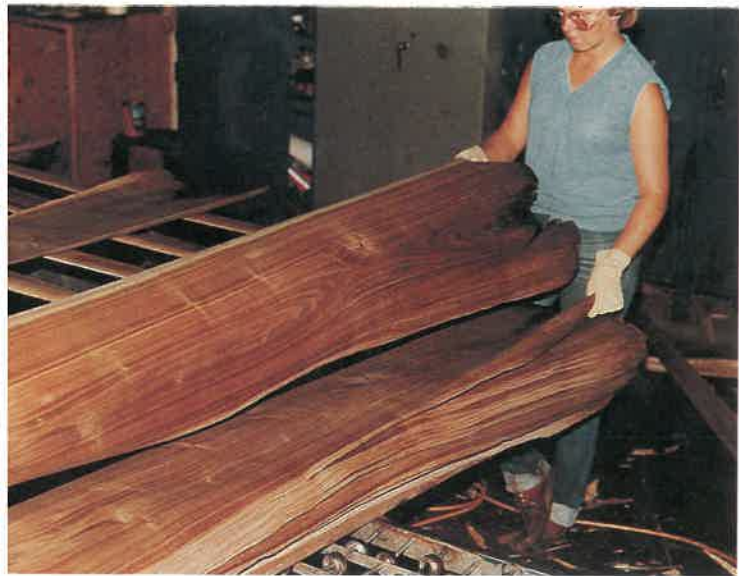
Fig. 35-36. Top. Slicing veneer. Flitch is clamped to machine table with hydraulic cylinders and moved up and down against a sharp knife. The machine operates at 80 strokes per minute. Veneer sheets are carried away on conveyor belts as shown. Bottom. Veneer plant worker stacks sheets of walnut veneer as they leave the end of the slicing machine. The veneer shown is 1/36 in. thick. (Bacon Veneer Co.)
