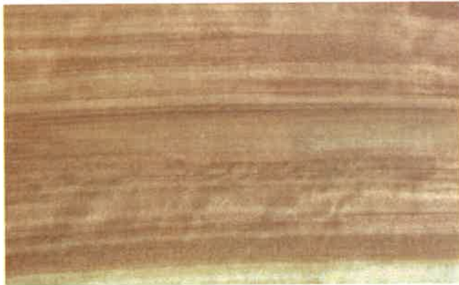
ASPEN. Soft, light, close-grained, and easy to work. White sapwood with light tan and brown streaked heartwood. Source: Europe, Western Asia and Middle Atlantic States. Used for furniture, and interior paneling.
