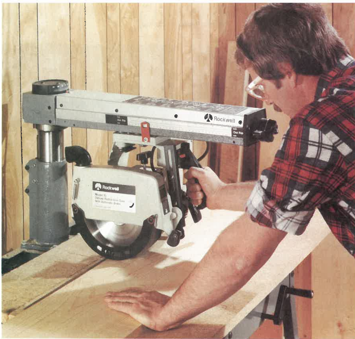
Fig. 3-14. This is the proper procedure for crosscutting stock on the radial arm saw. (Delta International Machinery Corp.)
