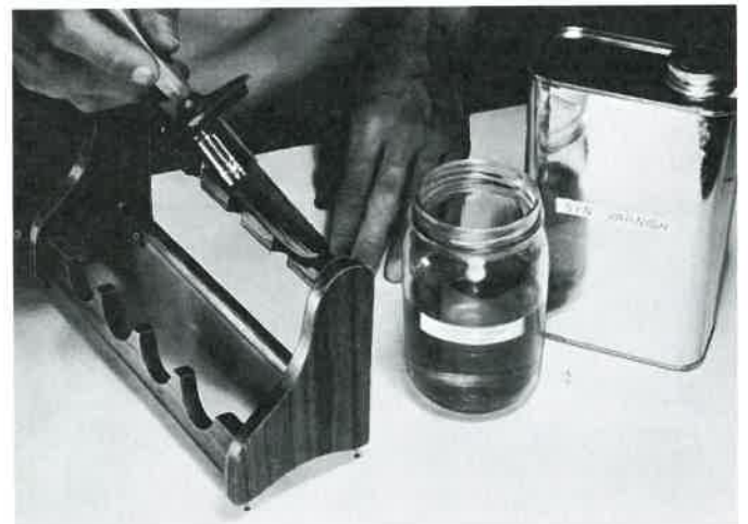
Fig. 12-43. Work supported on small nails driven into underside.
