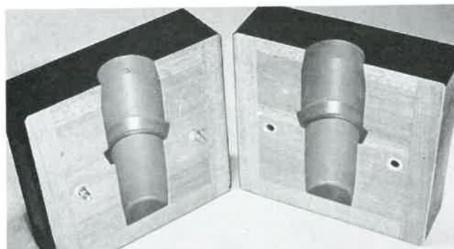
Fig. 32-22. This split core box forms a core with several different diameters. Note the brass dowel pins.
