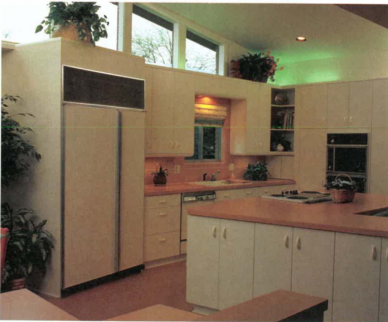
Fig. 24-1. The countertops in this kitchen are decorative and resistant to wear and scratching. Oil, grease, boiling water, and most household chemicals will not harm the surface.
