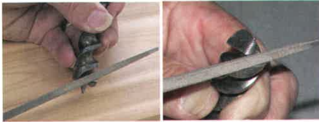
Fig. 6-3. Left. Filing the cutting lip. Right. Filing the spur. Try to maintain original bevel and do not file the outside.
