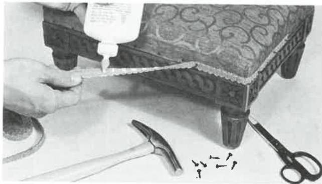
Fig. 25-26. Covering the tacked edge with gimp. Apply droplets of glue to the gimp and use temporary tacking to hold it in place until dry.
