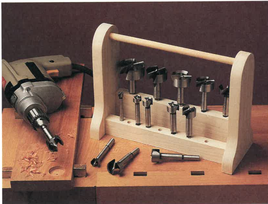
Fig. 6-16. Forstner bits produce a smooth, flat-bottomed hole. (Leichtung, Inc.)
