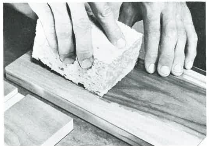
Fig. 11-14. Using moisture to raise the wood grain.
