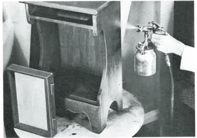
Fig. 12-58. Work set on a turntable in the spray booth. The wings of the air cap are in a vertical position to form a horizontal pattern as the gun is stroked up and down with the grain.
