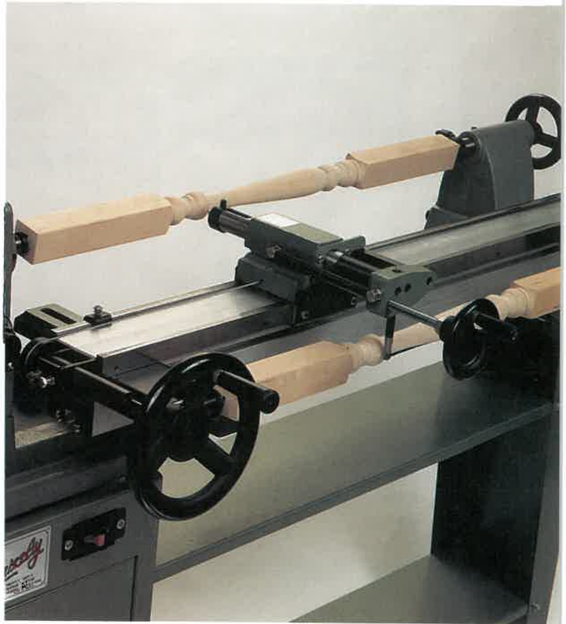
Fig. 33-20. General-purpose wood lathe with duplicator. (Grizzly Imports, Inc.)
