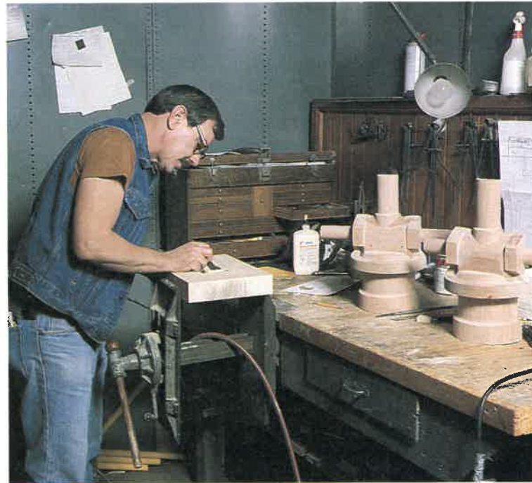
Fig. 32-23. Patternmaker prepares a core box for the split pattern shown on the bench. Note the special type of vise that will clamp and support the workpiece in a variety of positions. (Fisher Controls)
