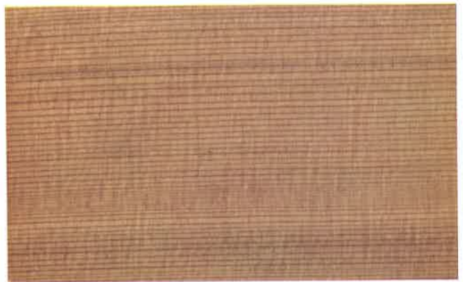
CEDAR, RED, WESTERN. A soft wood, light in weight (23 lbs. per cu. ft.). Similar to redwood except for cedar-like odor. Pronounced transition from spring to summer growth (see edge-grain sample). Source: Western coast of North America, especially Washington. Used for shingles, siding, structural timbers and utility poles.
