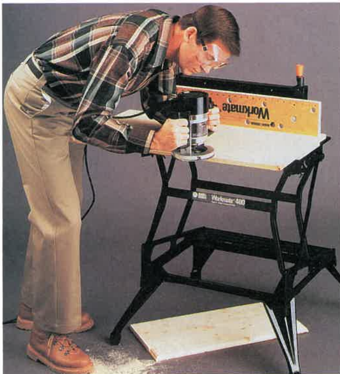
Fig. 3-27. The work is securely clamped and eye protection is being worn while operating the router. (Black & Decker)
