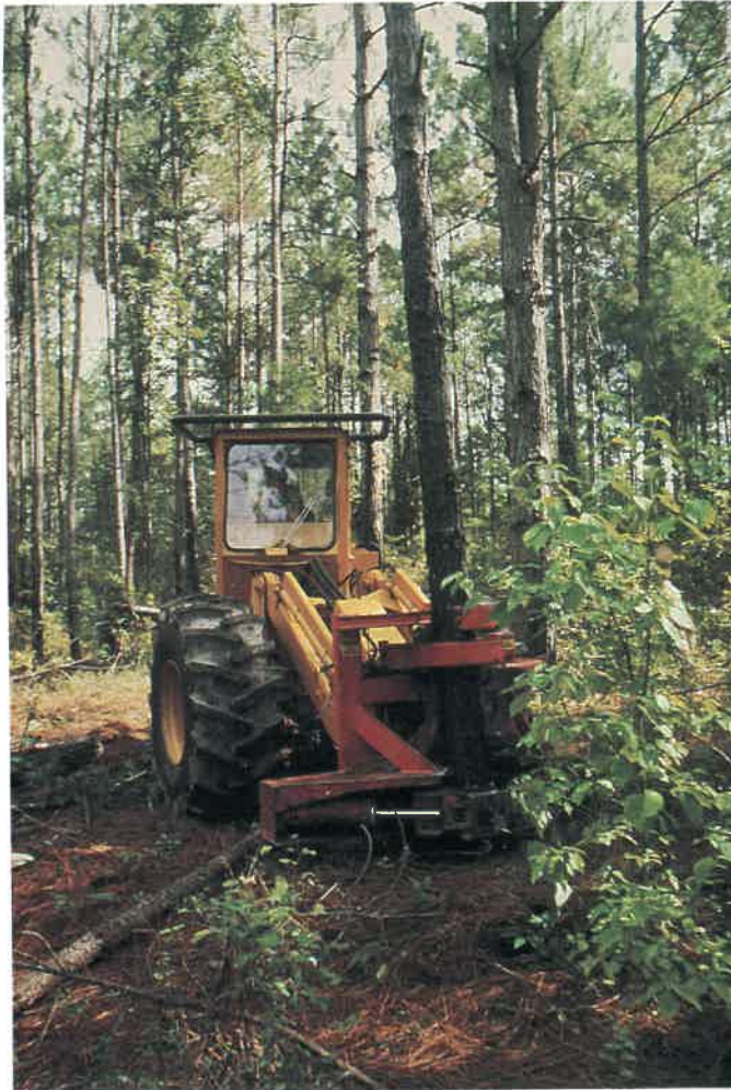
Fig. 35-20. The hydraulic unit mounted on the front of this tractor is capable of cutting trees several inches in diameter, and then laying the tree down in the desired location for trimming. (Southern Forest Products Association)
