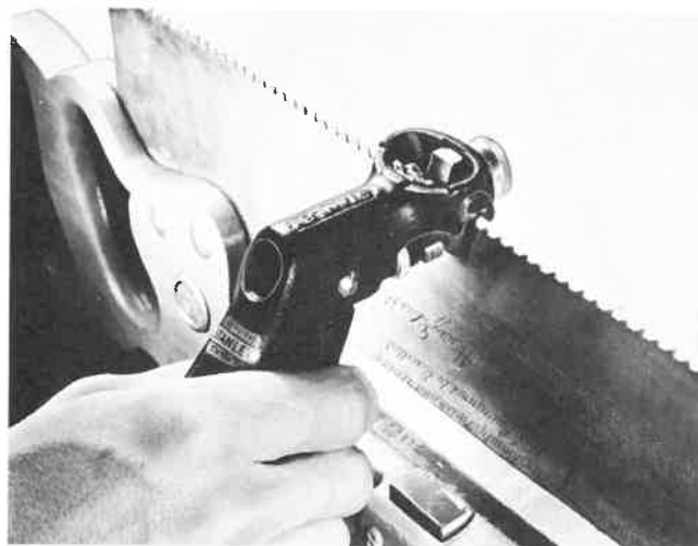
Fig. 4-24. Setting the teeth. In this position the saw set will bend the teeth away from you.
