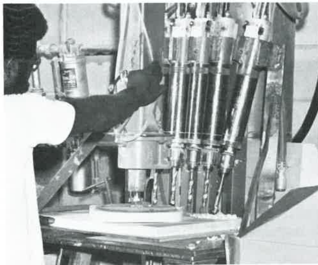
Fig. 16-39. Skilled operator adjusts air clamp on fixtured boring machine. Recommended operating pressure for the self-feed drilling units is 90 psi (621 kPa). (The ARO Corp.)
