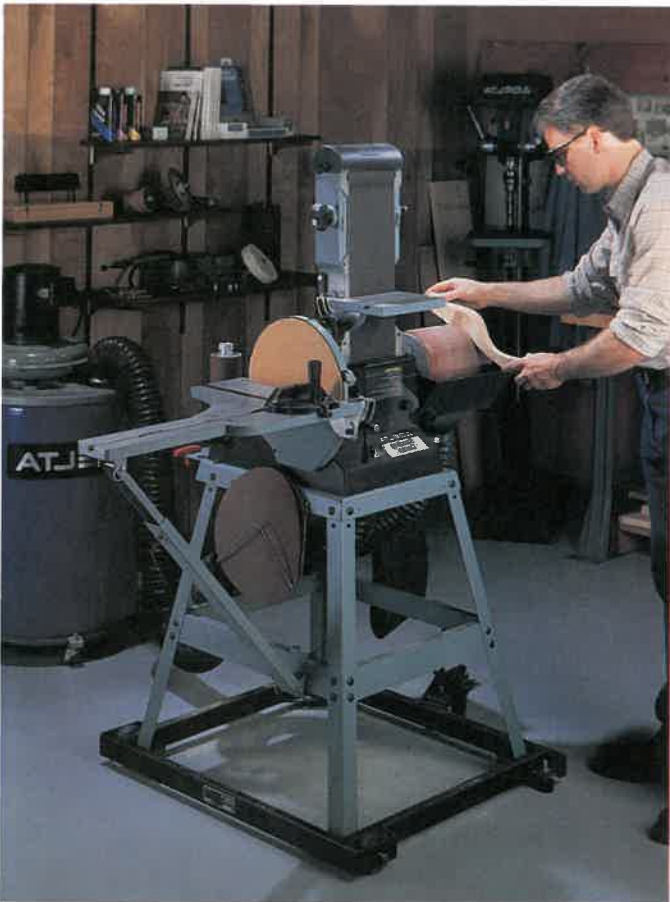
Fig. 33-19. Combination belt, disk, and drum sander in use. The dust collector helps extend the useful life of the machine. (Delta International Machinery Corp.)
