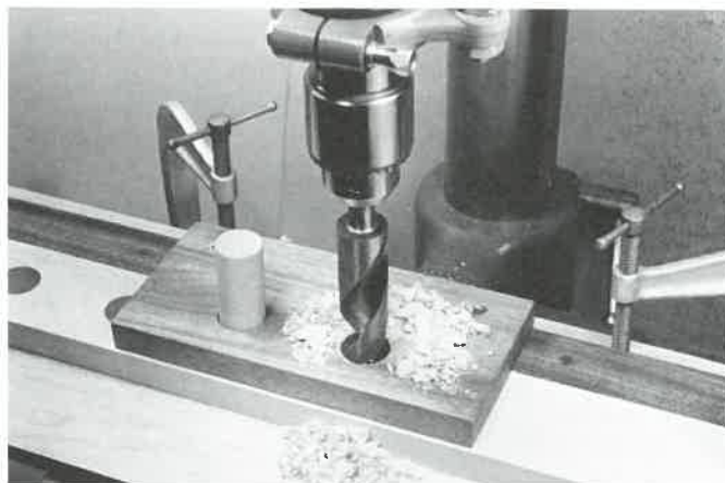
Fig. 16-16. Fixture for boring equally spaced holes. Taper the lower end of the dowel pin slightly so it can be easily slipped into the previously bored hole.
