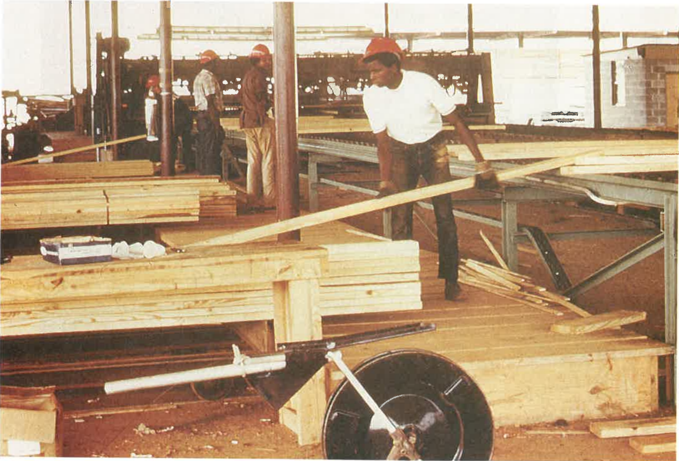
Grading southern yellow pine boards in a modern sawmill. (Southern Forest Products Association)
