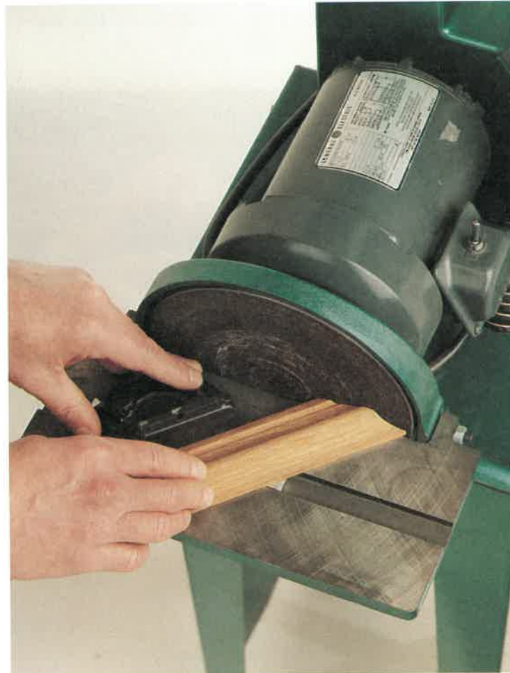
Fig. 7-40. The miter gauge may be used with a disk sander to modify or smooth a miter cut. (Foley-Belsaw Co.)
