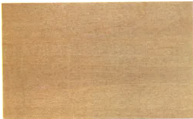
BASSWOOD. The softest and lightest (26 lbs. to cu. ft.) hardwood in commercial use. Fine, even texture with straight grain. Especially easy to work with hand tools and highly resistant to warpage. Heartwood is a light yellowish-brown. Used for drawing boards, food containers, moldings, woodenware and core stock for plywood.
