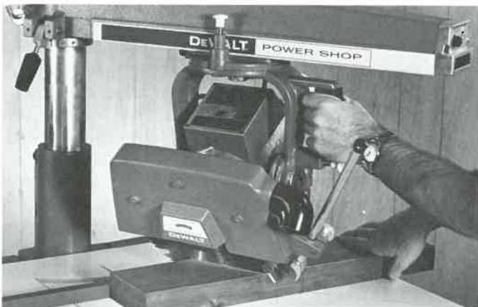
Fig. 14-64. Cutting a compound miter. Lower guard cannot be used.
