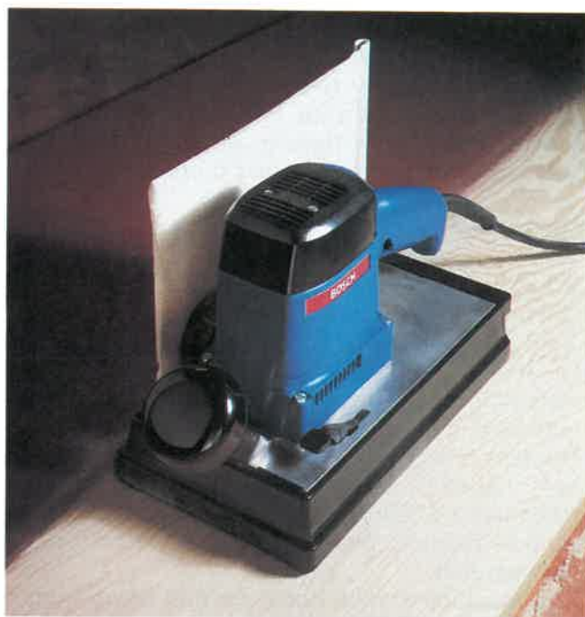
Fig. 33-13. This portable sander is being used to smooth a surface for finish. (Bosch Power Tool Corp.)
