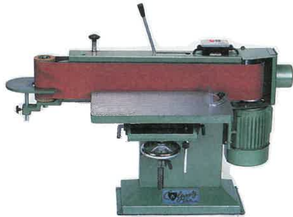
Fig. 19-36. A 6'' x 30'' edge sander. The sanding belt is mounted on two vertical drums; one a drive, the other an idler. The belt runs in a vertical plane while the workpiece is supported on a horizontal table during sanding. Edge belt sanders are used primarily to sand the edges of rectangular stock. (Grizzly Imports, Inc.)
