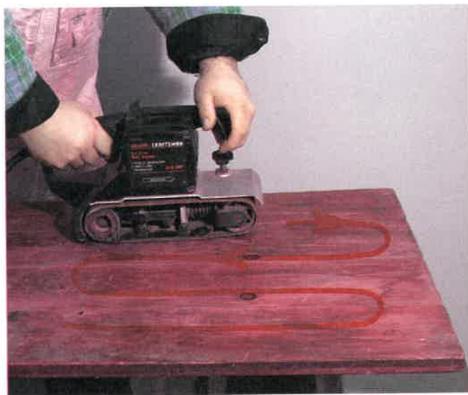
Fig. 19-19. Using belt sander. Note the direction of the sanding operation (arrow).
