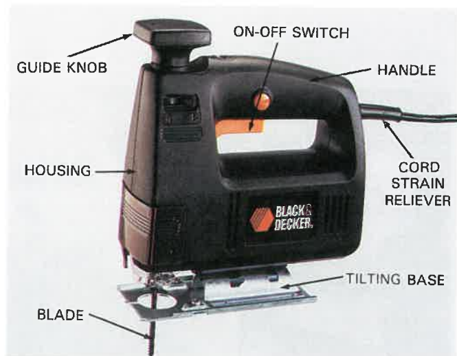
Fig. 15-36. Parts of a saber saw. (Black & Decker)
