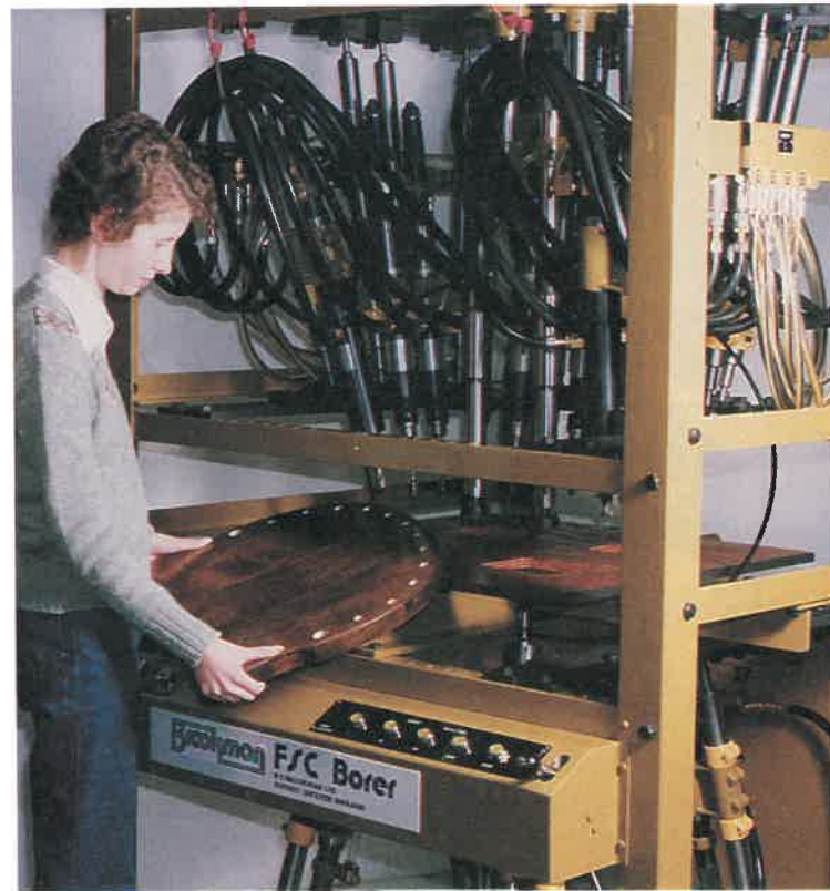
Fig. 16-40. This chair seat boring machine has 4 lower and up to 16 upper drilling heads, held in mounts which allow angling up to 30 deg. out of vertical. (R.S. Brookman, Ltd.)
