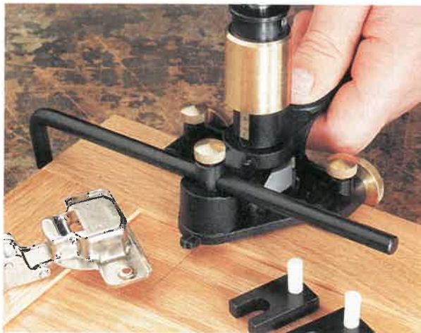
Fig. 21-15. Right. Drilling 35mm flap hinges. Left. Drilling standard 35mm hinges. (Veritas Tools, Inc.)
