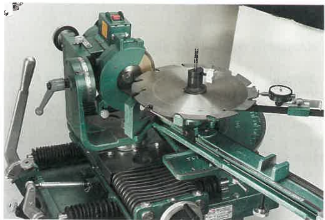
Fig. 14-12. Each tooth is individually ground to shape on a carbide blade. Top. Grinding the side. Bottom. Grinding the top. (Foley-Belsaw Co.)
