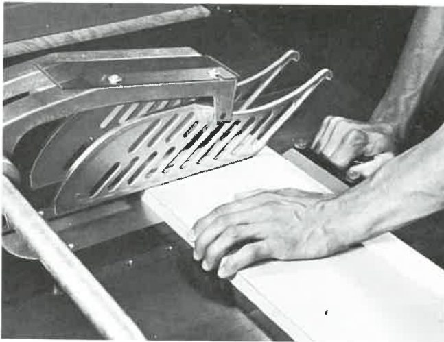
Fig. 14-23. Cutting duplicate lengths using stop rod. Guard can be used for this, but has been removed to show this operation.
