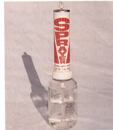
Fig. 12-66. A small, self-powered spray unit can be loaded with spray materials used by a regular gun.
