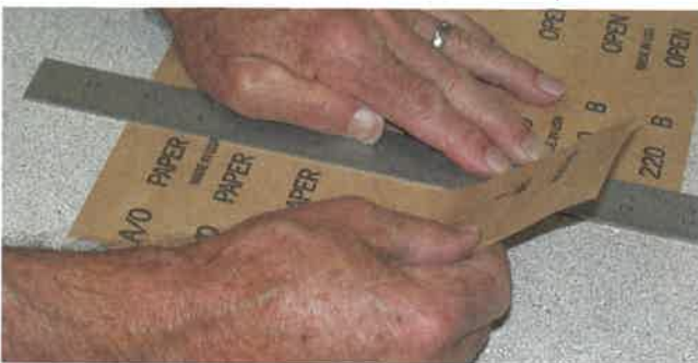
Fig. 11-9. Tearing a sheet of abrasive paper into smaller pieces.
