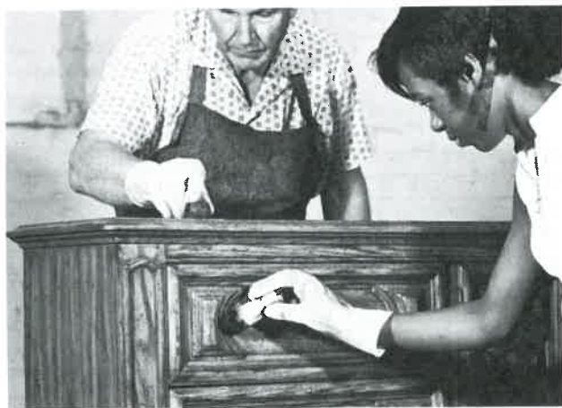
Fig. 12-20. Skilled workers wipe glaze-coated surfaces to produce highlights and special effects. (Thomasville Furniture Industries, Inc.)
