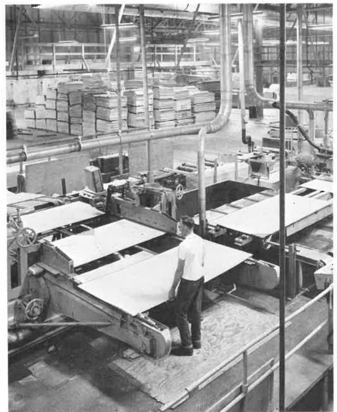
Fig. 35-34. Double-end machines trim the plywood panels to exact width and length.
