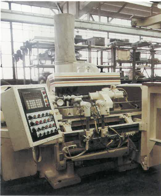
Fig. 17-43. This automatic turning lathe handles stock up to 4 in. (101.5 mm) square and 42 in. (1.06 m) long. The cutterhead turns at a speed of 2700 rpm. The feed chute and front cover are opened to show the basic mechanism. (Mattison Machine Works)
