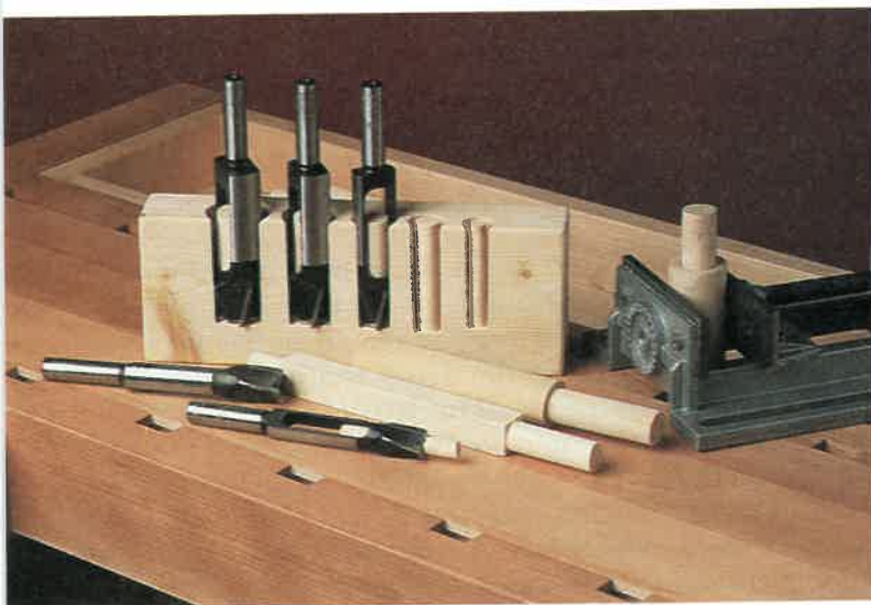
Fig. 7-27. A plug cutter may be used to make standard size plugs and round tenons. (Leichtung, Inc.)
