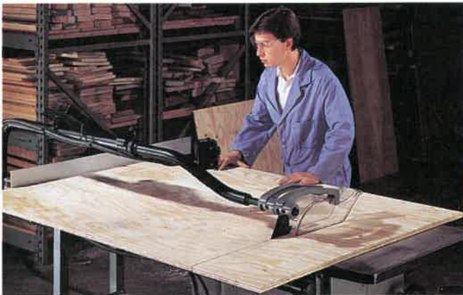
Fig. 3-11. This student woodworker is using the guard and splitter in a safe manner. (Delta International Machinery Corp.)
