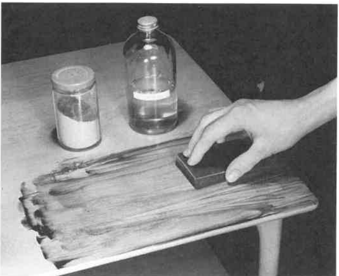
Fig. 12-45. Top. Materials for polishing a finish. Bottom. Rubbing a final coat with rottenstone and oil. Felt pads that have been used for a coarse abrasive should not be used for a fine abrasive.
