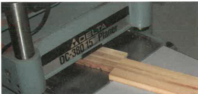
Fig. 13-31. Butt the ends of short pieces together. They also can be turned at a slight angle to provide a smoother feed.
