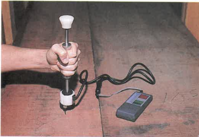
Fig. 2-9. Top. Modern digital moisture meter. LEDs indicate correct moisture percentage. Middle. Probes inserted into end cut. Bottom. Hammer probe provides readings up to 1 inch below surface. (Forestry Suppliers, Inc.)
