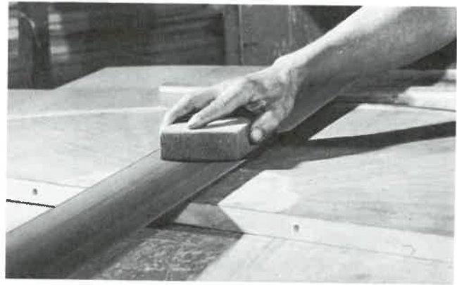
Fig. 19-28. Finish sanding with a hand stroke belt sander. Belt is No. 150 aluminum oxide abrasive on an E weight paper backing. (Norton Co.)
