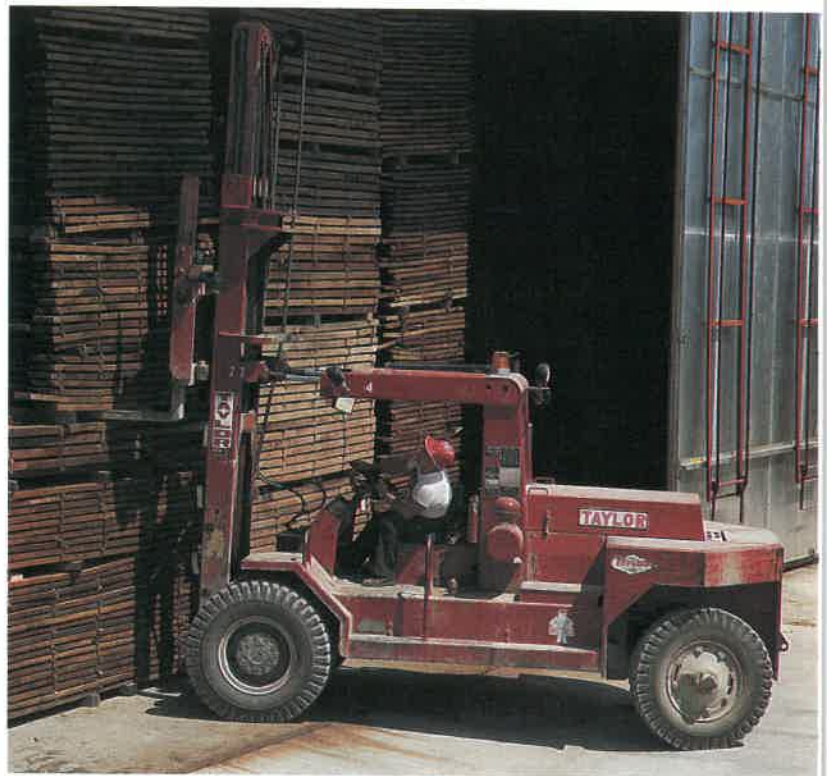
Fig. 35-11. Large kilns are used to season lumber at a sawmill. Note the "stickers" that separate the layers. (Kimball International)
