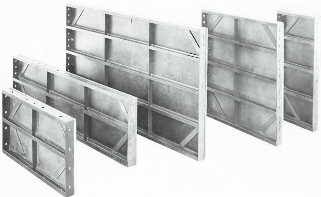
Fig. 26-22. Modular form components are produced in several sizes (dimensions are in feet): 2 x 2, 2 x 4, 4 x 2, 4 x 4, 8 x 2, and 8 x 4. Plywood facing (3/4 in.) is attached to a steel frame. (Symons Corp.)
