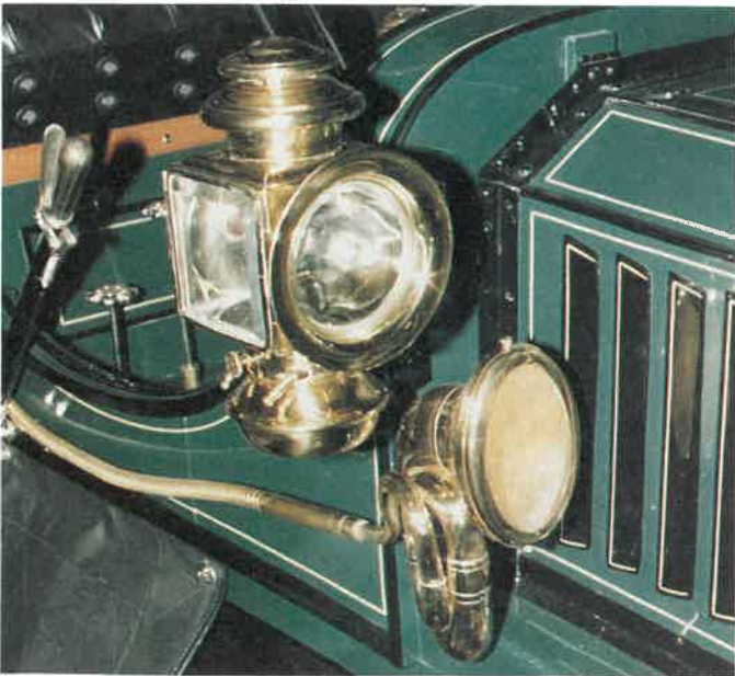
Fig. 12-27. The finish on this wood car body was produced with several coats of lacquer. Each coat was rubbed before the next one was applied.
