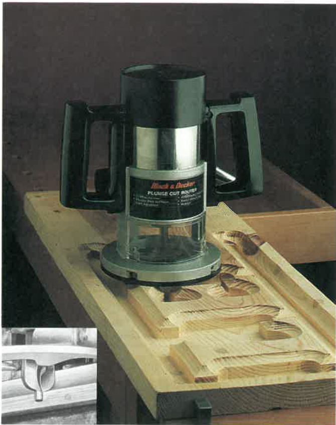
Fig. 18-11. The pilot tip shown in the inset guides the router along the edges of the grooves in this sign. (Leichtung, Inc.)
