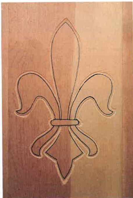
Fig. 20-15. Outlining a design with the V-tool.
