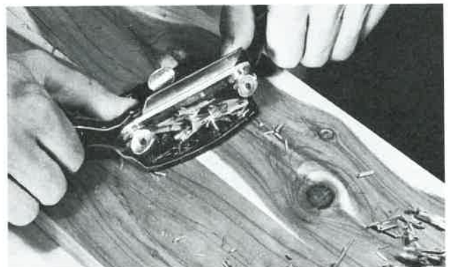
Fig. 11-21. Using the cabinet scraper.
