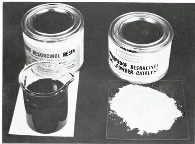
Fig. 9-7. Resorcinol-formaldehyde resin glue.
