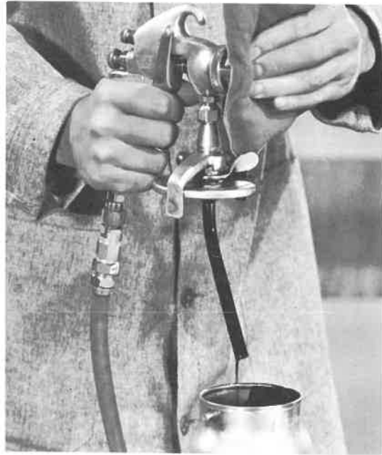
Fig. 12-62. Forcing material from the gun back into the cup. (DeVilbiss Co.)
