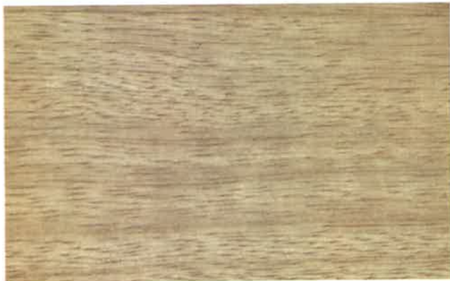
LIMBA. A light blond wood from the Congo, often sold under the trade name Korina. It has an open grain with about the same texture and hardness of Mahogany. Works easily with either hand or machine tools. Used for furniture and fixtures, especially where light tones are required.
