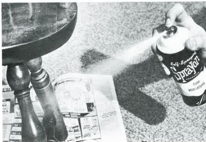
Fig. 12-65. Using a spray can for touch-up work. (Sprayon Products Inc.)
