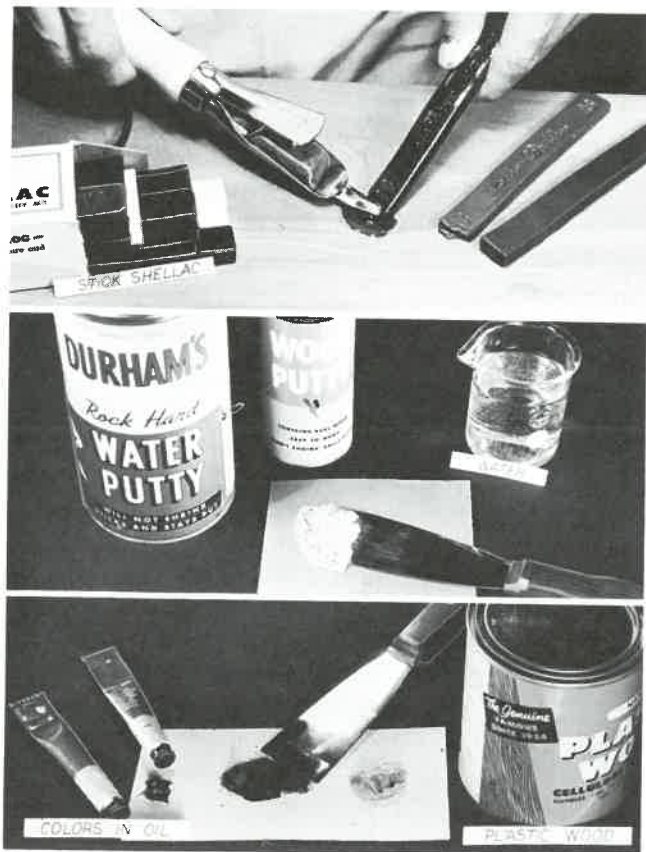
Fig. 11-23. Repairing a wood surface. Top. Melting stick shellac into the defect with a burn-in knife. Center. Wood putty is easy to mix and use. Bottom. Adding color to natural shade of plastic wood.
