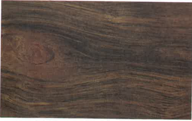
PALDAO. A fairly hard wood with large pores that are partially plugged. Grain patterns are striking and beautiful and provide an excellent example of an "exotic" wood. Source: Philippine Islands. Sometimes selected by architects for special fixtures or built-ins for public or institutional buildings.
