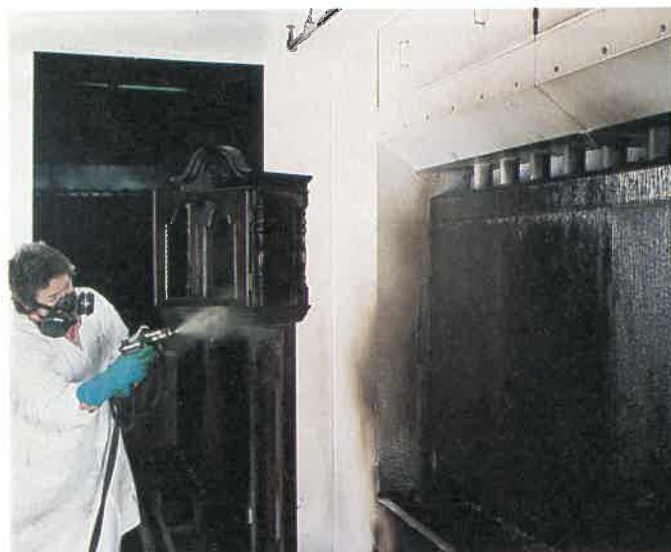
Fig. 12-47. A glaze coating is applied in an industry spray booth. An advanced air washer design helps trap the glaze overspray before it reaches the outside atmosphere. (DeVilbiss Co.)
