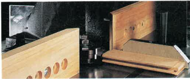
Fig. 18-37. Using a miter gauge to shape the end of a panel frame. (Freud, Inc.)
