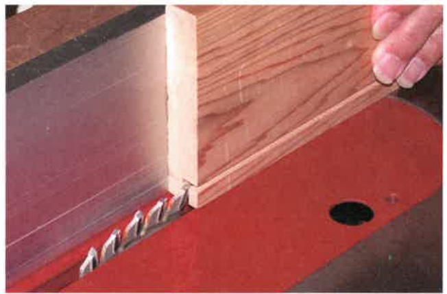
Fig. 3-13. The guard may not be used in this operation and, therefore, should be approved by the instructor.
