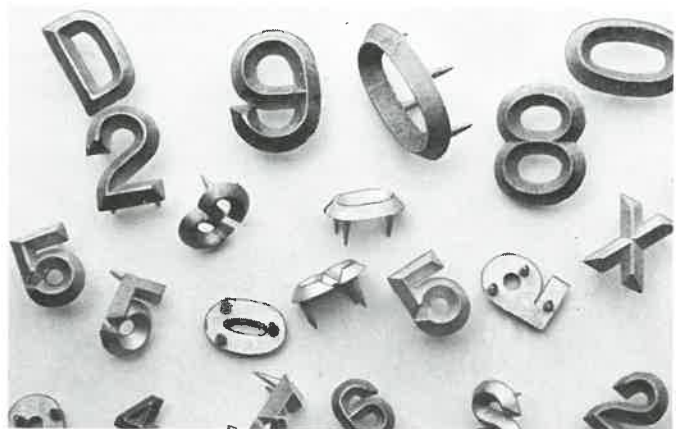
Fig. 32-5. Pattern letters and figures are used for identification purposes. Some have spurs or pins that are driven into the wood. Those with a plain back are cemented in place.
