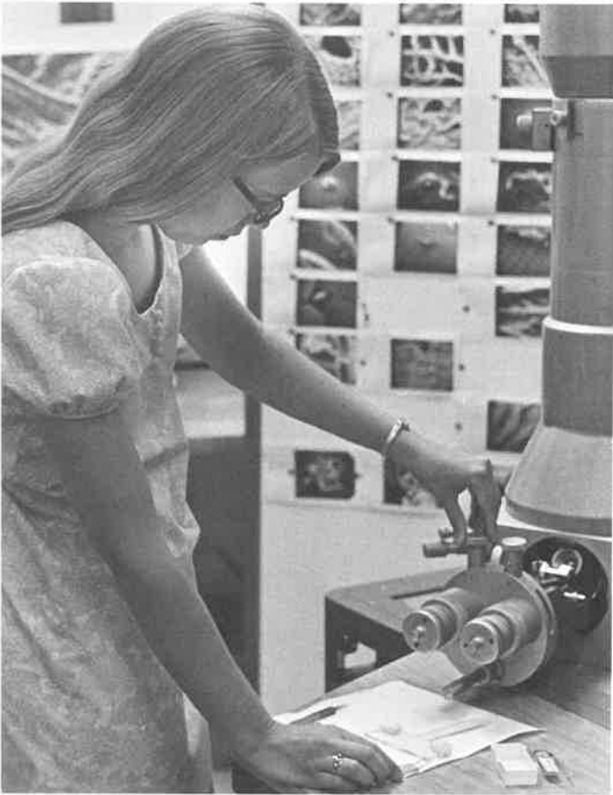
Fig. 36-15. Technician uses electron microscope to probe wood's fine structure. Microscope is capable of providing a magnification of 100,000X. (Forest Products Laboratories)
