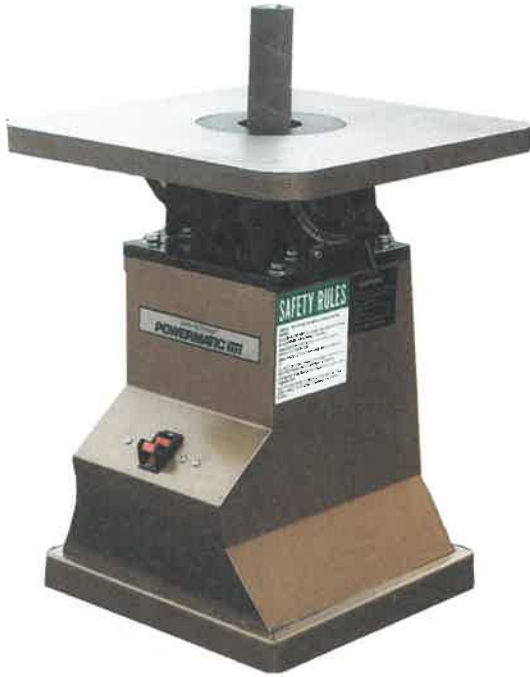
Fig. 19-34. This oscillating single spindle sander has a table with tilting capabilities. (Enlon Import Corp.)
