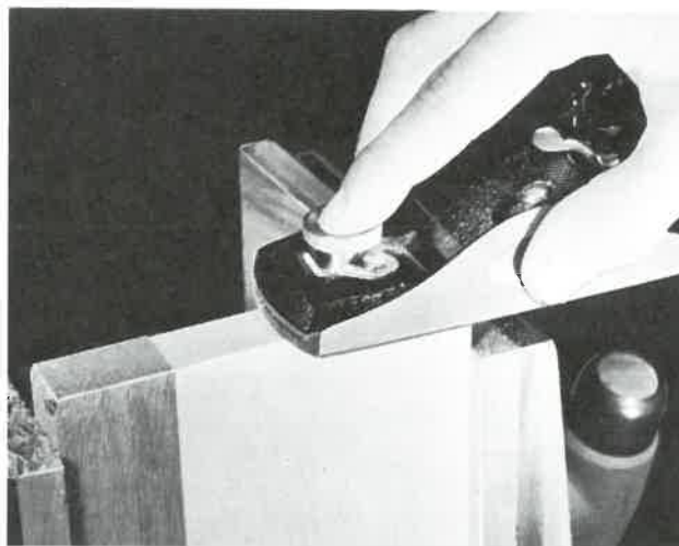
Fig. 5-25. Planing end grain. The edge is supported with scrap stock.
