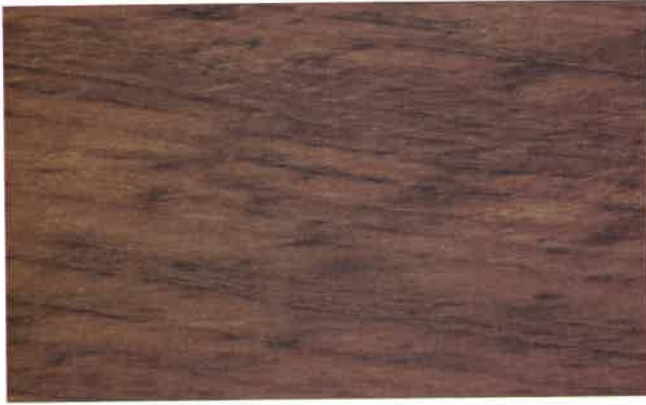
OAK, ENGLISH. Open-grained with a texture similar to regular oak. Light tan to deep brown color with dark spots that create an unusual figure and grain character. Source: England. Used for fine furniture and special architectural woodwork.
