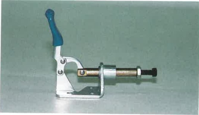
Fig. 9-24. Straight-line toggle clamps provide a pulling or pushing action. (Te-Co)
