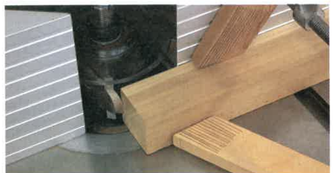
Fig. 3-29. Hold-downs help to make a smooth, safe cut on the shaper.
