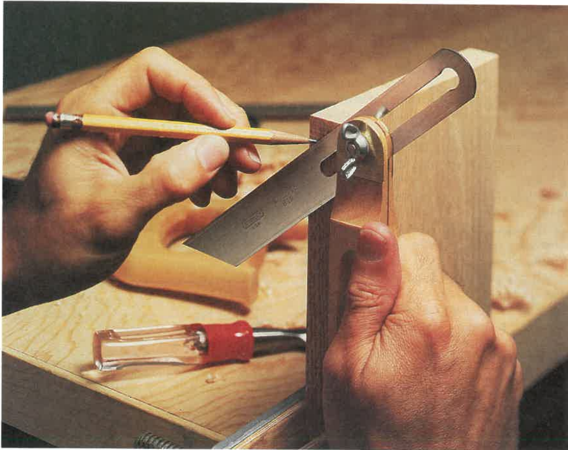
Fig. 7-36. Using the T-bevel square to mark a miter cut. (The Stanley Works)
