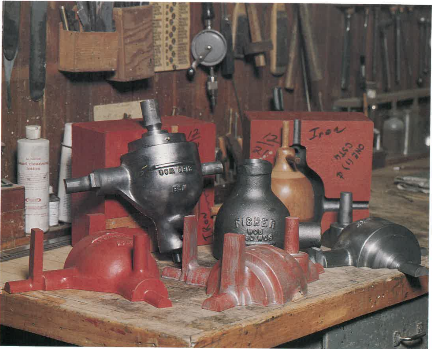
Finished casting of a valve body (center) surrounded by master and production patterns used in the foundry process. (Fisher Controls)
