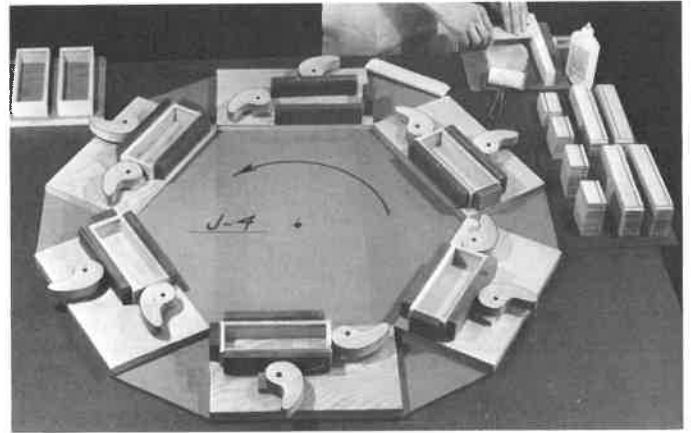
Fig. 34-26. Gluing setup for assembly of sides and ends. The polyvinyl glue makes an initial set in the time required for the subassembly to travel around the turntable.
