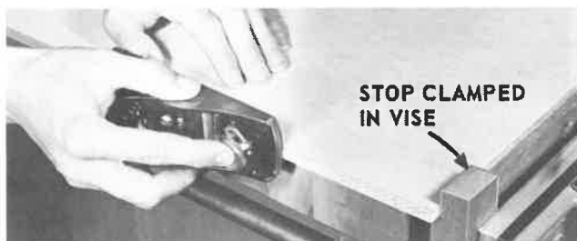
Fig. 5-27. Using block plane to smooth edge of plywood.
