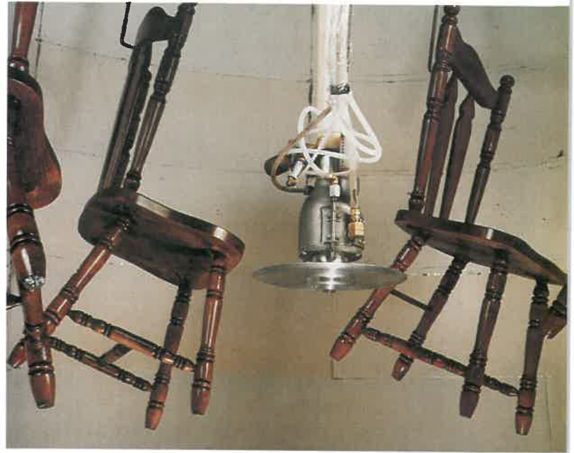
Fig. 12-69. Industrial electrostatic painting equipment applying the final coat to these chairs. A conveyor carries the work past the painting unit. (Ransburg Electrostatic Equipment)
