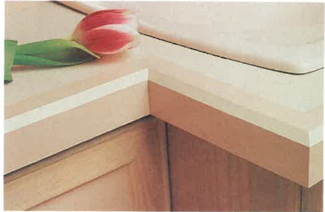
Fig. 24-17. Solid surface materials, though more expensive than traditional high-pressure plastic laminates, produce nice renewable surfaces. Solid surface materials are 1/2 in. thick and do not require a substrate. (Wilsonart)
