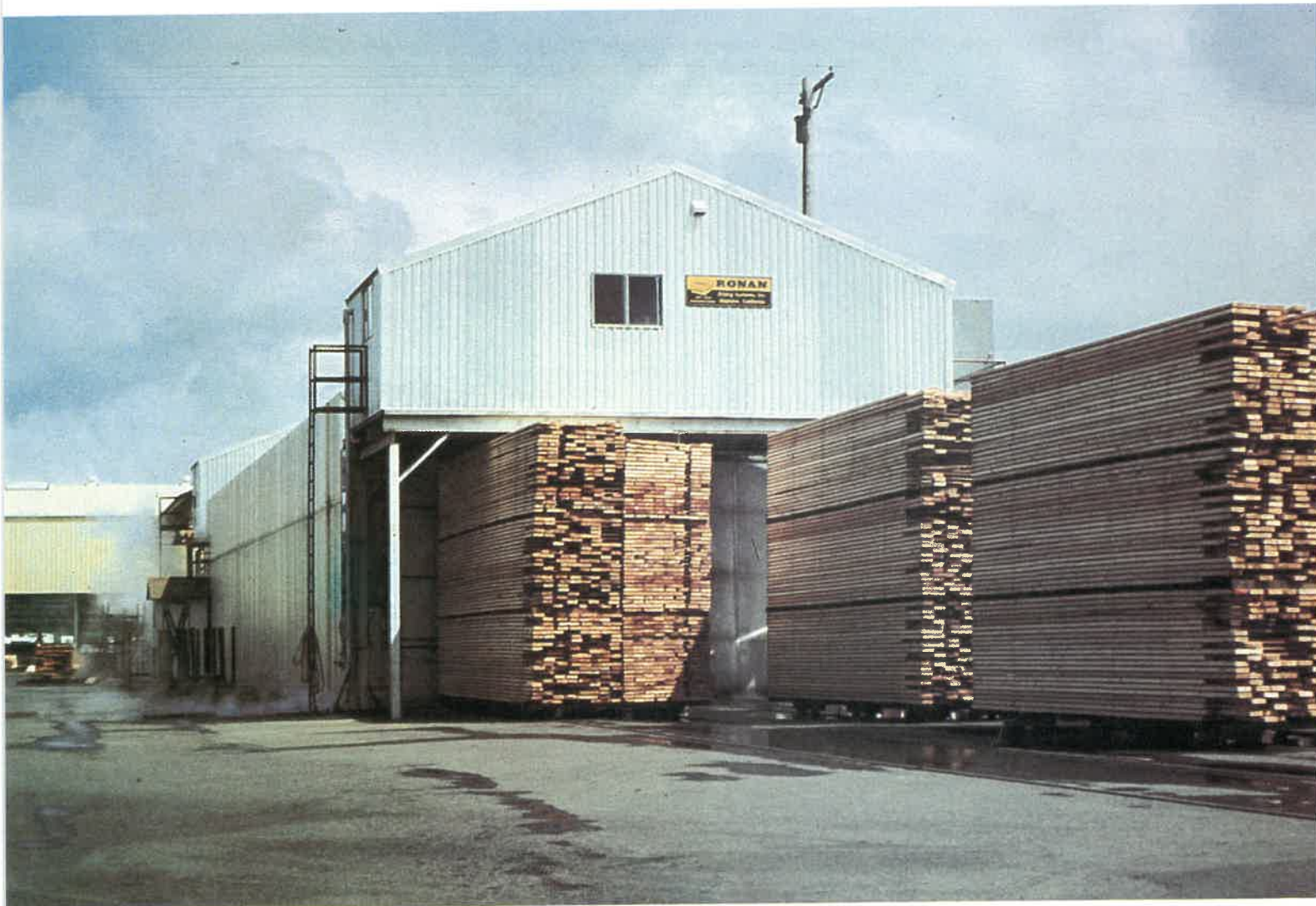
Fig. 2-8. Kiln drying lumber in large quantities. (Forest Products Laboratory)
