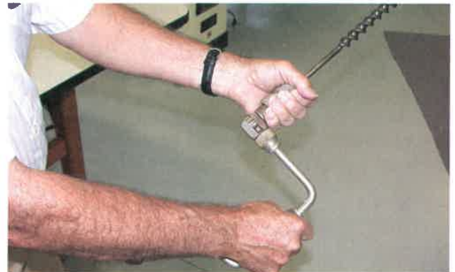
Fig. 6-5. Tightening the chuck of the brace by holding the shell and turning the handle.
