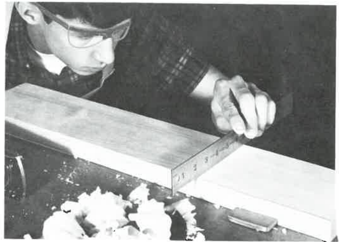
Fig. 5-12. Checking the surface. The rule or straightedge must be placed diagonally across the stock to reveal twist (wind).
