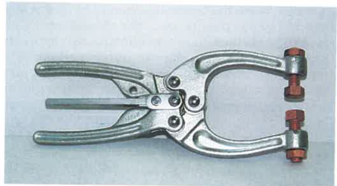
Fig. 9-26. Squeeze-action toggle clamps are sometimes called toggle pliers. They are generally used where C-clamps might be used. (Te-Co)
