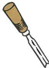
Fig. 8-24. Shaping an inside contour with an outside ground gouge.
