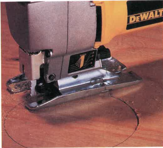
Fig. 4-18. Cutting plywood with a saber saw. (DeWalt)
