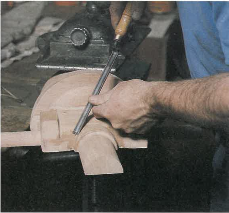
Fig. 32-9. Final work on pattern in an industrial plant. A patternmaker must be highly skilled in the use of hand tools. (Fisher Controls)
