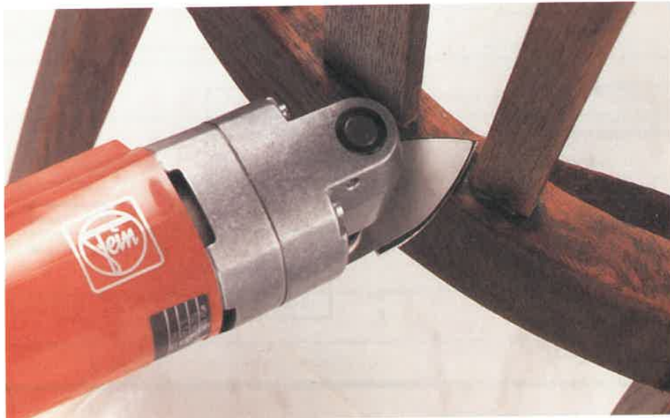
This detail sander can reach into spaces not previously accessible by power sanders. (Fein Power Tools Inc.)
