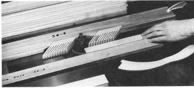
Fig. 34-22. Precision planing stock to width on the shaper. Ring guard has been removed for this photo.
