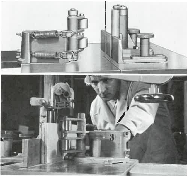
Fig. 15-22. Top. Resawing attachment. Bottom. Resawing attachment in operation. (Northfield Foundry and Machine Co.)
