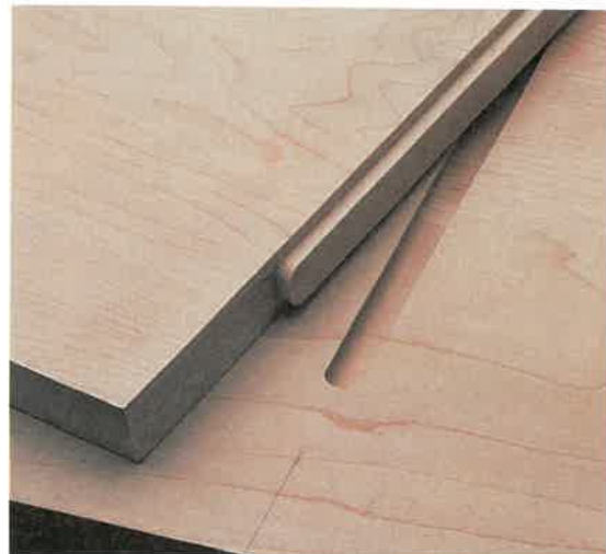
Left. Varying the spacing of dovetails adds interest to the project. Right. Sliding dovetails are particularly suitable for fitting shelves and partitions. (Leigh Industries, Ltd.)
