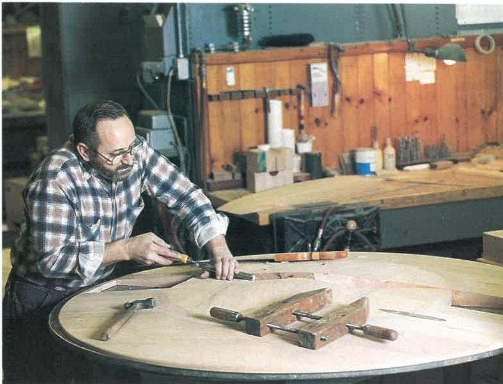
Fig. 36-11. Patternmaker using a gouge to form a curved surface on a large circular pattern. (Fisher Controls)
