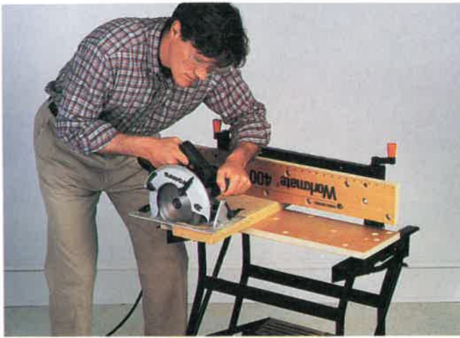
Fig. 3-16. Notice that the base of the saw is resting on the stock as the blade is moved forward, the work is securely clamped, and the operator is using both hands to hold the saw. (Black & Decker)
