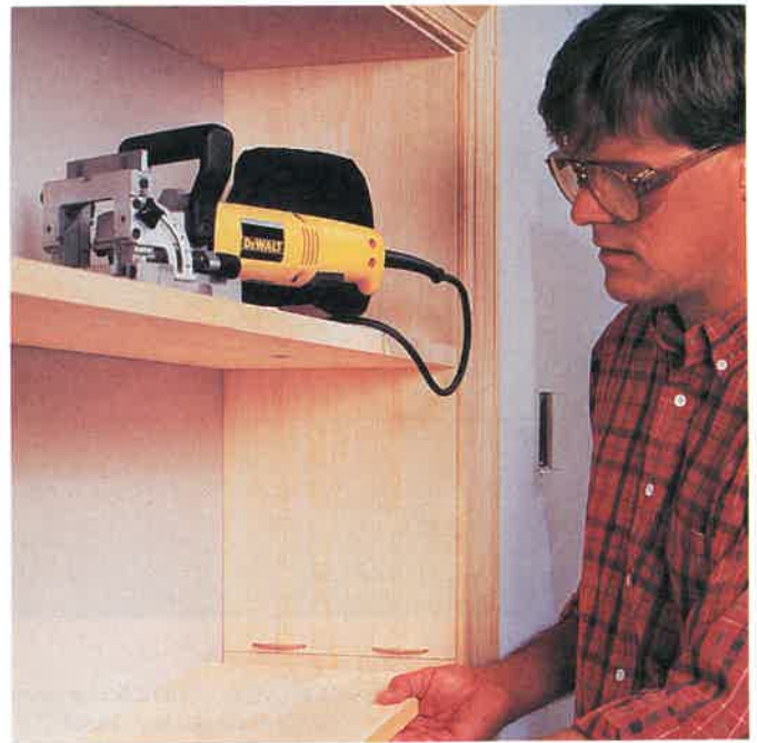
Fig. 7-46. Plate joinery may be used in the place of dowel or dado joints. (DeWalt)
