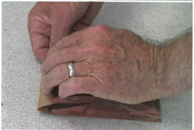
Fig. 11-10. Attaching abrasive paper to rubber sanding block. Top. Place one edge of paper in jaw, abrasive side up. Center. Stretch across bottom of block. Bottom. Place other end in jaw. Be sure paper is properly aligned before closing jaws.
