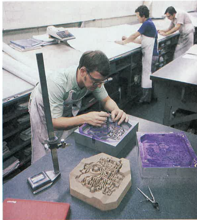
Left. Patternmaker completing work on original wood pattern for an engine block. View shows a special tool being used to form a fillet around the base of a core print. Right. Patternmaker inspecting metal core box for an air-cooled engine head. Sample core is shown in foreground. Workers in background are checking full-sized pattern drawings. (Lear Siegler)
