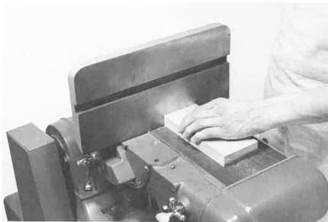
Fig. 19-9. Sanding a flat surface. Belt travel is toward the table which serves as a stop.
