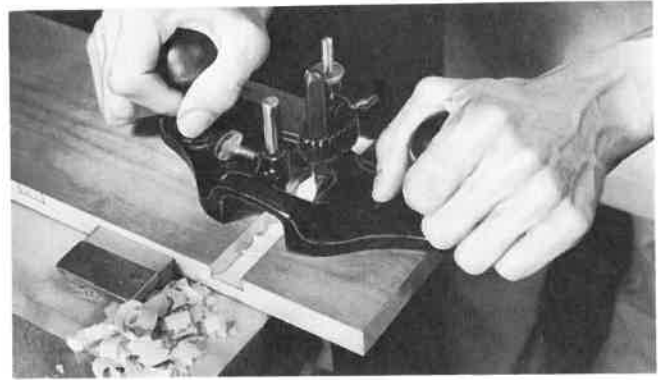
Fig. 7-9. Using a router plane to smooth the bottom of a dado joint.
