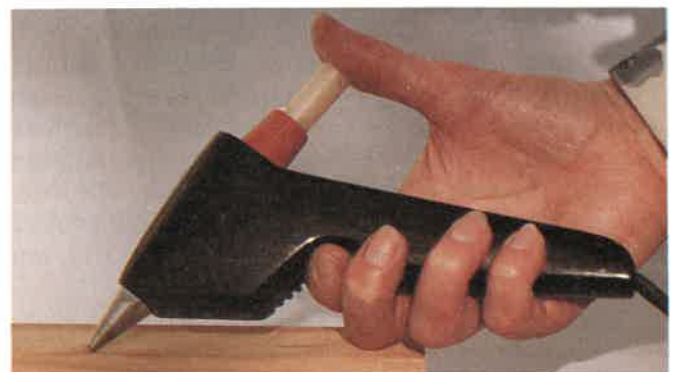
Fig. 9-4. Hot melt glues are applied using a special applicator, in this case, a glue gun.
