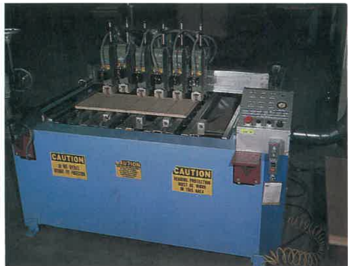
Fig. 34-2. A specialized setup for cutting several fine grooves in a panel at once. Each piece cut in this manner will be exactly the same. (Campbellrhea Mfg., Inc.)
