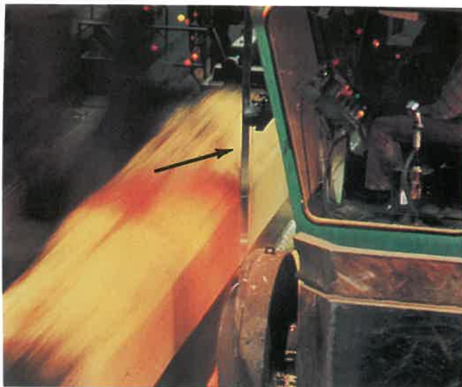
Fig. 35-24. Operator (called a sawyer) seated at control console of headrig. High speed bandsaw blade (arrow) produces slabs, timbers, and large rectangular pieces called "cants." (John Walker)
