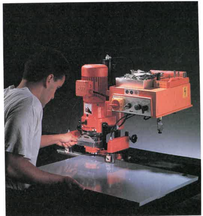
Left. Surface mounted and flush mounted RTA (Ready To Assemble) fittings for cabinets and furniture. Right. This "minipress" is basically a drill press with 5 spindles that is specifically designed to bore holes for press-in hardware. (Julius Blum, Inc.)
