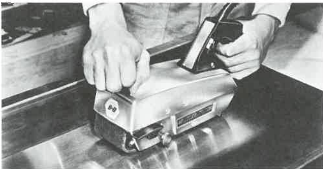
Fig. 19-20. Using a portable belt sander to polish a lacquer finish. Operation requires nylon fabric belt, special abrasive, and a skilled woodworker. (Black & Decker)
