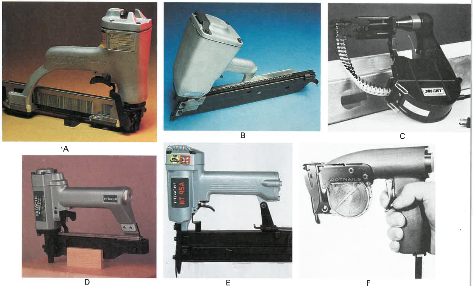
Fig. 10-28. Tackers, staplers, and nailers. A—Medium duty air-powered staple gun. B—Heavy duty air-powered power nailer. (Paslode Co., Div., of Signode) C—Self-feeding screw system. D—Narrow crown finish stapler. (Hitachi Power Tools) E—Finish nailer that uses .18 gauge brads. (Hitachi Power Tools) F—Air tacker. Holds up to 5,000 staples in one cartridge. (Spotnails, Inc.)
