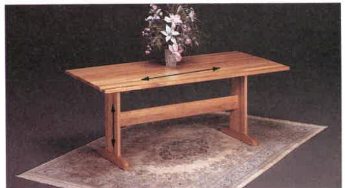
Fig. 21-18. Grain direction in solid wood construction. (Period Furniture, Inc.)
