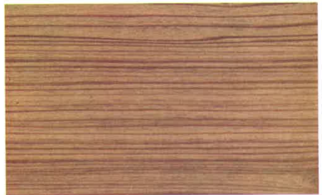
CYPRESS. Light in weight, soft and easily worked. Fairly coarse texture with annual growth rings clearly defined (sample shows edge grain). Source: Southeastern Coast of the United States. Noted for its durability against decay. Used for exterior construction and interior wall paneling.
