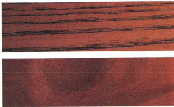
Fig. 12-25. These two surfaces were finished with medium-oil varnish over 25 years ago. They are still beautiful, with no cracks or chips.
