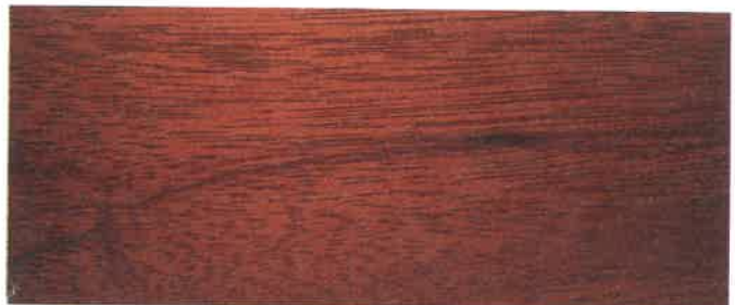
Fig. 12-11. This photo shows the surface of mahogany. It generally has large pores that require filler to obtain a smooth surface.
