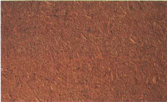
Fig. 35-42. Close-up view of a particle board panel surface. The flakes are still visible even though the surface is smooth.
