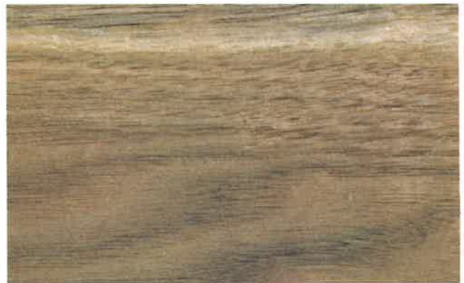
BUTTERNUT. Fairly soft, weak, light in weight (27 lbs. to cu. ft.), with a coarse texture. Grain patterns resemble walnut. Large open pores require a paste filler. Works easily with hand or machine tools. Sometimes used for interior trim, cabinetwork, and wall paneling.
