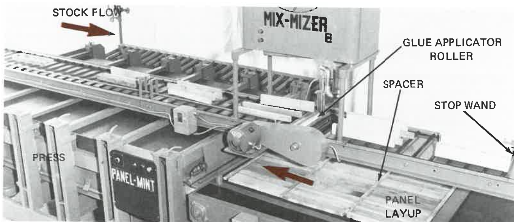
Fig. 9-42. Modern edge gluing machine for lumber 5/8 in. to 2 in. (16 mm to 51 mm) thick. Conveyor carries stock over glue applicator and stops when pieces contact the stop wand. Operator takes stock from top conveyor and lays up panels. When load is complete, it is moved into press by lower conveyor. Steam heated platens are pressed against the panel surfaces by air bags and edge pressure is supplied by air cylinders. Joints cure while operator lays up next load. (James L. Taylor Mfg. Co.)
