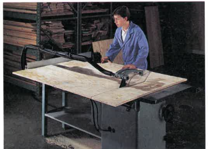
Fig. 14-74. Making a cut across the grain. (Black & Decker)
