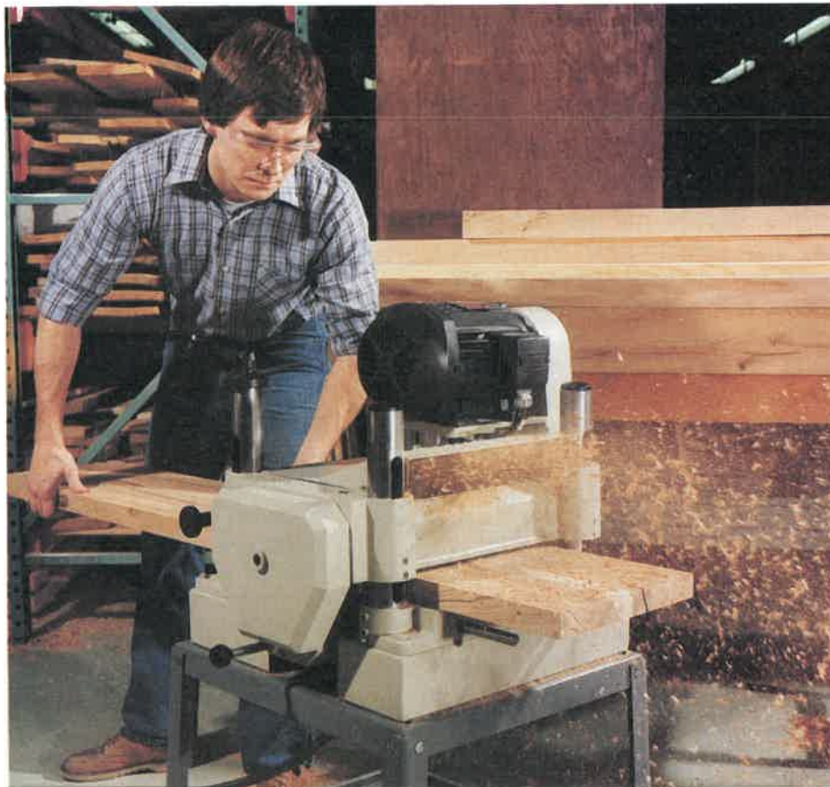
Fig. 13-29. Stand to the side when feeding stock into the planer. (Delta International Machinery Corp.)
