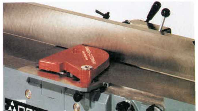
Fig. 3-7. This jointer is fitted with a proper guard. Be sure that it works smoothly and it is in place for safe operation.
