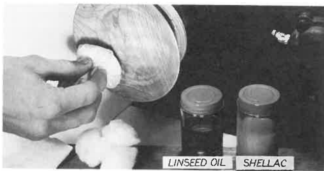
Fig. 17-31. Applying a French polish.
