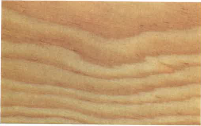
PINE, PONDEROSA. Lightweight (28 lbs. to cu. ft.) and soft. Straight grained and uniform texture. Not a strong wood but works easily and has little tendency to warp. Heartwood is a light reddish-brown. Change from springwood to summerwood is abrupt. Used for window and door frames, moldings, and other millwork; toys, models.
