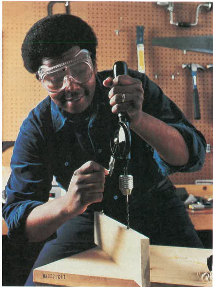
Fig. 6-18. A hand drill is useful for drilling small holes. (The Stanley Works)
