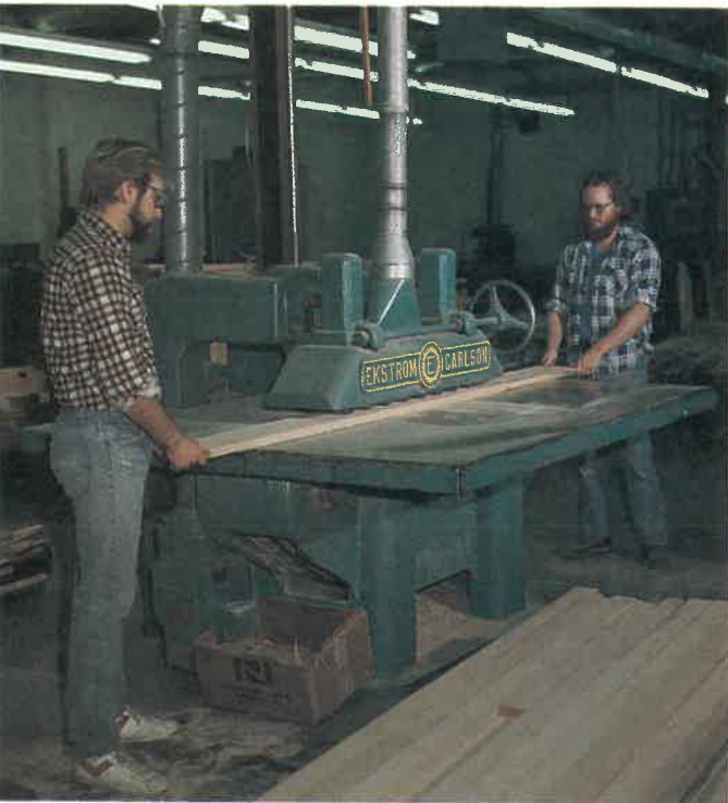
Fig. 14-81. When using a straight line rip saw, the fence is not required. Power feeder moves material through cut in straight line. (Campbellrhea Mfg., Inc.)
