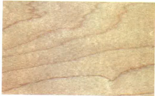
MAPLE, SUGAR. Also called Hard Maple. It is hard, strong, and heavy (44 lbs. to cu. ft.). Fine texture and grain pattern. Light tan color, with occasional dark streaks. Hard to work with hand tools but machines easily. Is an excellent turning wood. Used for floors, bowling alleys, woodenware, handles, and quality furniture.
