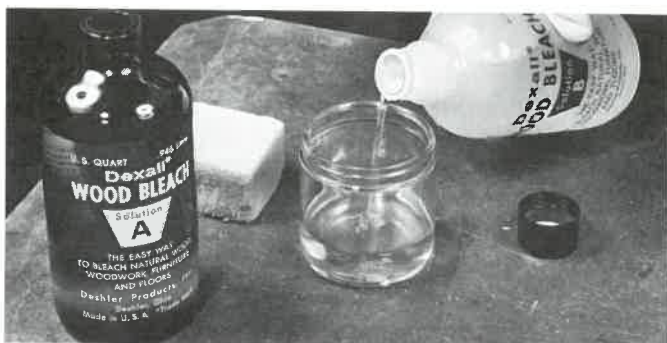
Fig. 12-10. Mixing a commercial wood bleach. Note that the worker is wearing rubber gloves. (Sherwin-Williams Co.)
