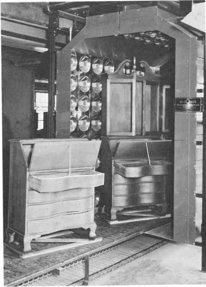
Fig. 12-80. Large pieces of furniture moving into a radiant heated oven on a floor-based conveyor. (Dry Clime Lamp Corp.)
