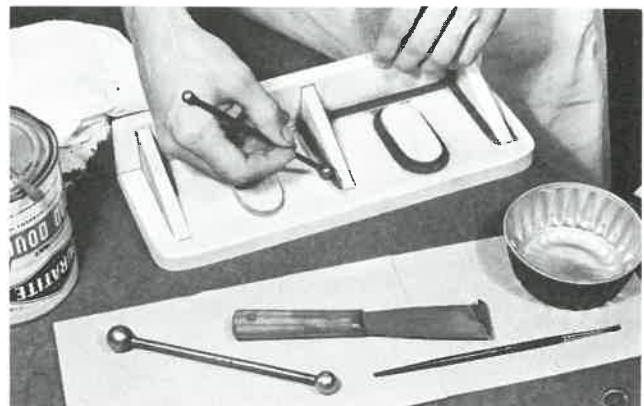
Fig. 32-12. Using a special plastic wood for fillet material. It is smoothed with a fillet iron dipped in lacquer thinner.
