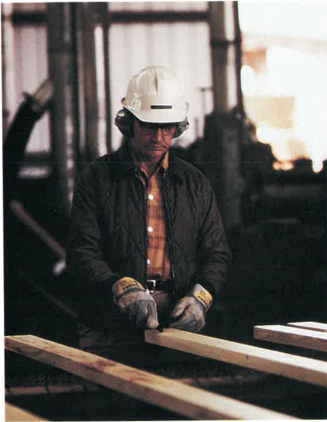
Fig. 35-26. Grading boards as they come from the trimmer saws. (Southern Forest Products Association)
