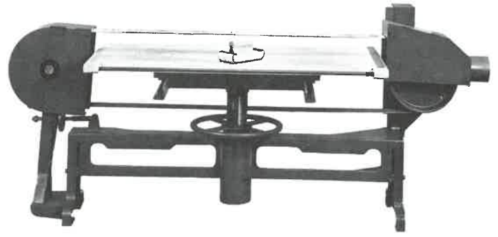
Fig. 19-27. Heavy-duty belt sander with rubber faced drums. Notice that the abrasive belt is facing in, toward the drums. (Oliver Machinery Co.)
