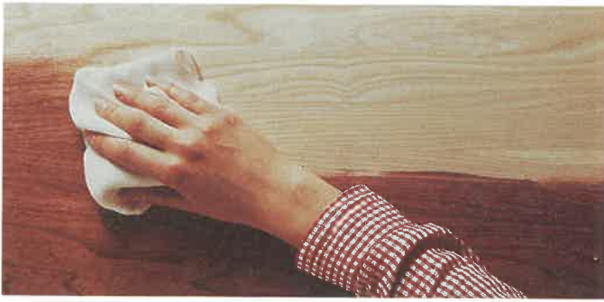
Fig. 12-18. Applying an oil base stain with a cloth. Do not allow the stain to dry before it is wiped. Wipe with the grain to remove the excess. (Deft, Inc.)
