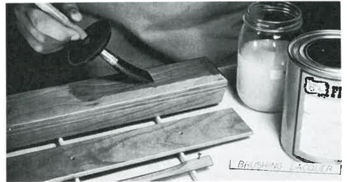
Fig. 12-42. Coating bottom surfaces first.
