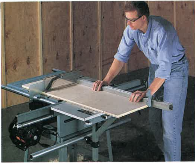
Fig. 14-2. This table saw has a tilting arbor and movable table. (Delta International Machinery Corp.)
