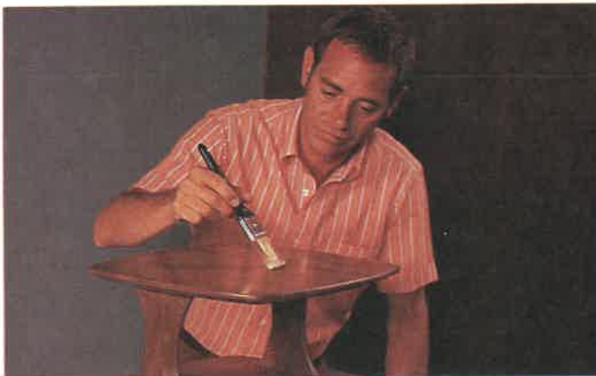
Fig. 12-40. Brushing finish coat. (Deft, Inc.)
