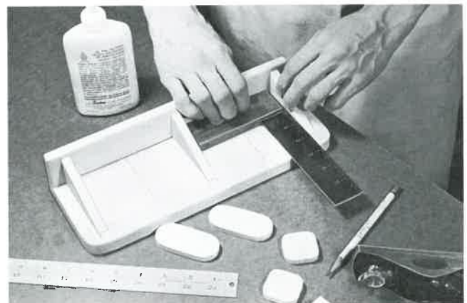
Fig. 32-8. Assembling a pattern with glue.
