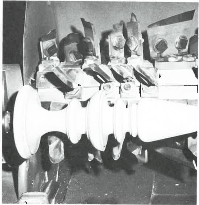
Fig. 17-44. Close-up of a cutterhead assembly. This assembly is used to produce lamp bases. (Forest City Tool Co.)
