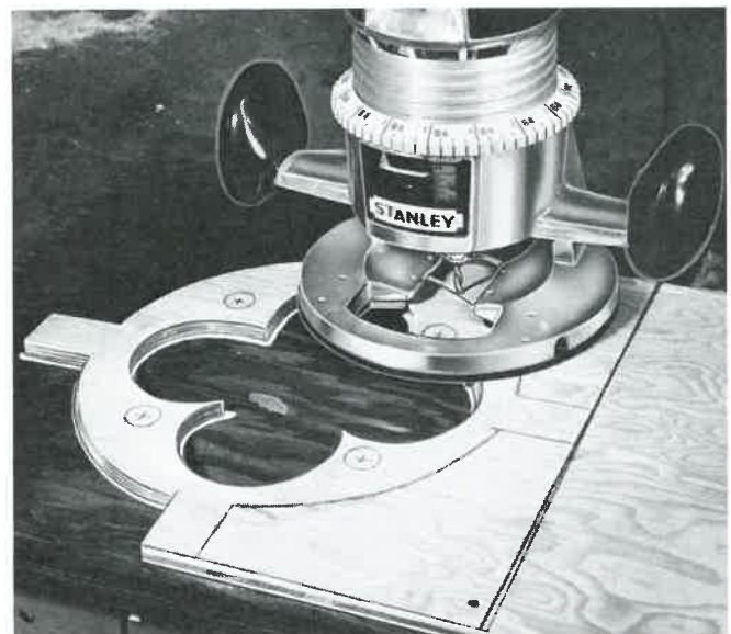
Fig. 18-10. A template for routing.
