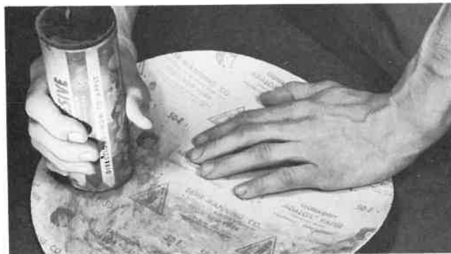
Fig. 19-3. Applying adhesive to a sanding disk.
