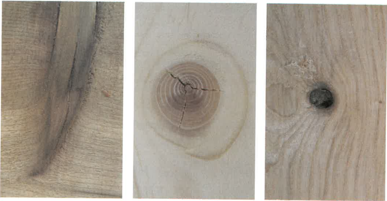
Fig. 2-4. Common kinds of knots. Left. Spike. Center. Intergrown. Right. Encased. The encased knot will probably loosen and fall out. (Forest Products Laboratory)
