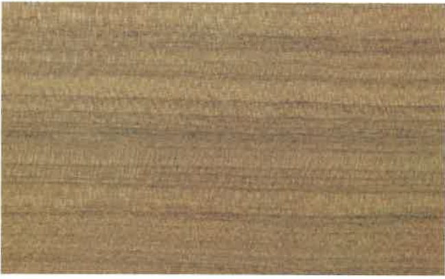
BELLA ROSA. Moderately hard, heavy and coarse textured. Striped and mottled grain patterns. Source: Philippine Islands. Available in veneer and lumber. Sample shows quartered veneer.
