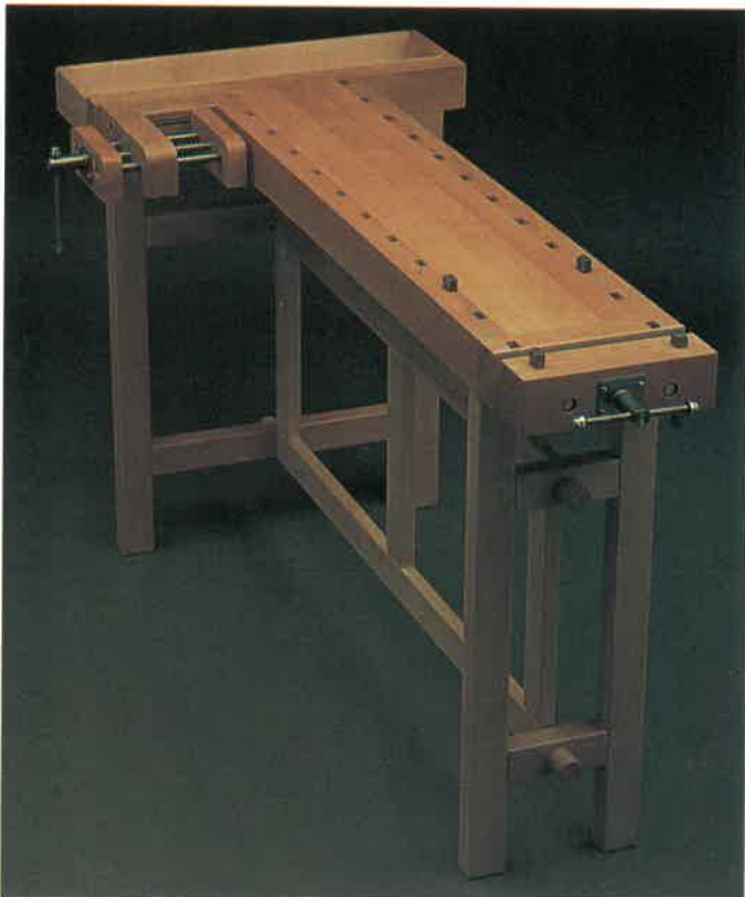
Fig. 33-8. This woodworking bench is equipped with two bench vises to handle most any job. (Leichtung, Inc.)
