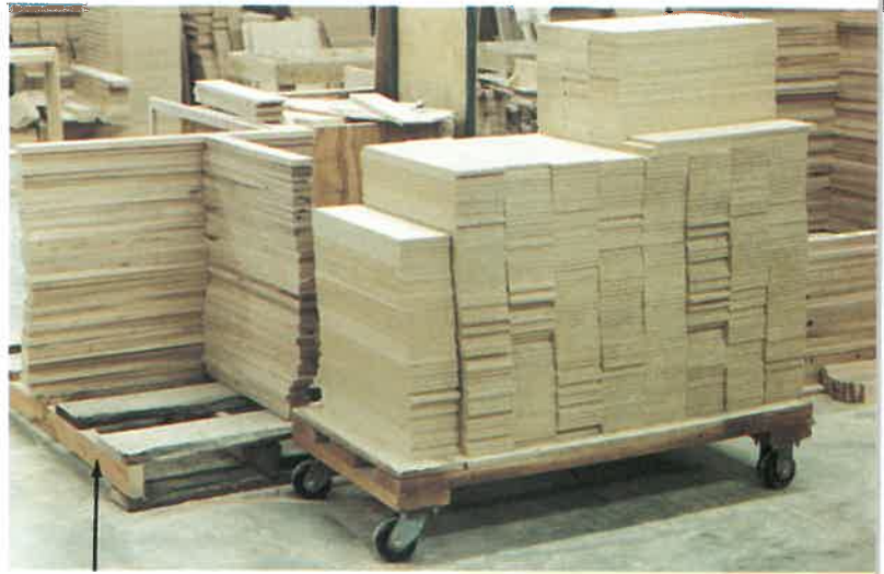
Fig. 34-16. Cabinet drawer parts stacked on stock cart for easy movement to machine stations. Partially assembled frames are stacked on a pallet (arrow) that is usually moved by a fork-lift truck. (Bertch Wood Specialties)
