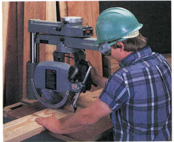
Fig. 14-61. Crosscutting with lower guard in position. Antikickback fingers are raised about 1/4 in. above the work. (Delta International Machinery Corp.)
