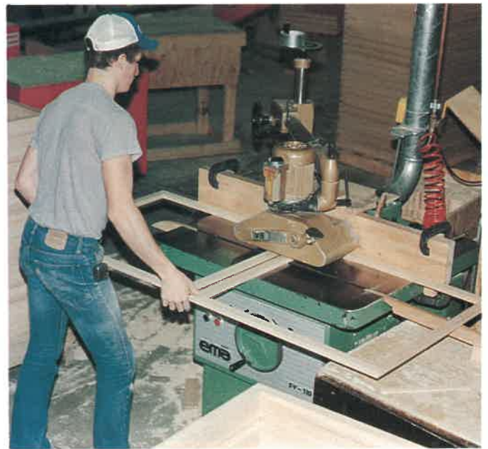
Fig. 36-9. Skilled worker checks the setup on a shaper with power feed mechanism. (Bertch Wood Specialties)
