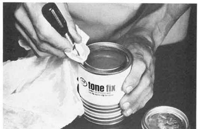
Fig. 12-38. Be sure to wipe out lip before closing container.
