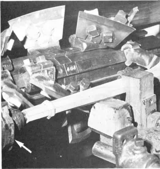
Fig. 17-45. Octagonal turning produced by cam action (arrow) varies depth of cut as workpiece rotates.
