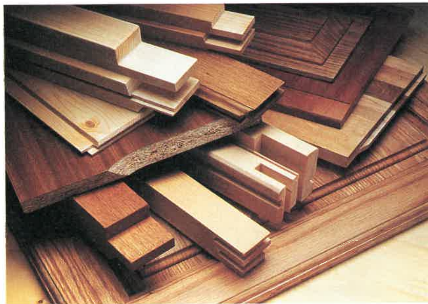
Top. This drilling assembly includes pneumatic drive and electric motor drive unit heads, mounted on framework built from Easi-rig System. (R.S. Brookman, Ltd.) Bottom. Typical work pieces of a modern double-end tenoner. (Wadkin PLC)
