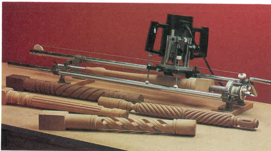
Fig. 18-17. A router with a jig was used to cut the grooves and spirals on these lathe turnings. (Leichtung, Inc.)
